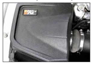
11. Install the K&N badge onto the lid and then install the lid onto the air filter housing as shown.
