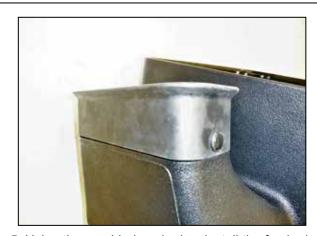
5. Using the provided push pins, install the fresh air intake hood seal onto the K&N air filter housing.
