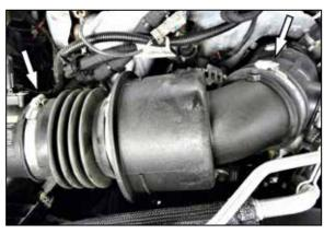
2. Loosen the two hose clamps securing the factory intake hose and then remove the hose from the vehicle.
