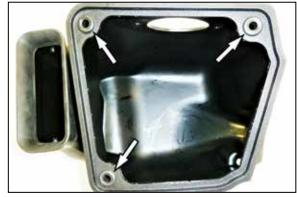
6. Install the three provided grommets into the K&N air filter housing as shown.
