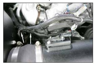
16. On 2014 and later model year vehicles that the electrical connection lays flat, it will be necessary to cut the electrical tape that secures the MAF pigtail to the main harness. Then pull approximately two inches of the MAF pigtail harness out from the main harness and retape the harness covering This will allow enough slack in the harness to allow connection.
