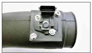
14. Install the mass air sensor assembly into the K&N intake tube and secure with the provided hardware. Be sure to install the sensor in the correct direction as shown. NOTE: 2024 model year vehicles and later have a different mass air sensor, the connector lays flat as compared to the sensor pictured.
