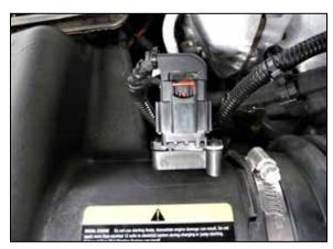
3. Disconnect the mass air sensor electrical connection. NOTE: 2024 model year vehicles and later have a different mass air sensor, the connector lays flat as compared to the sensor pictured.
