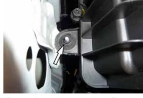
4. Remove the nut that secures the air filter housing into the vehicle and then lift up and remove the air filter housing from the vehicle.
