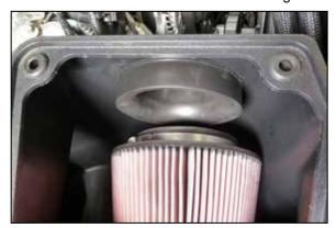
9. Install the filter adapter into the filter housing and secure with the provided hardware.
