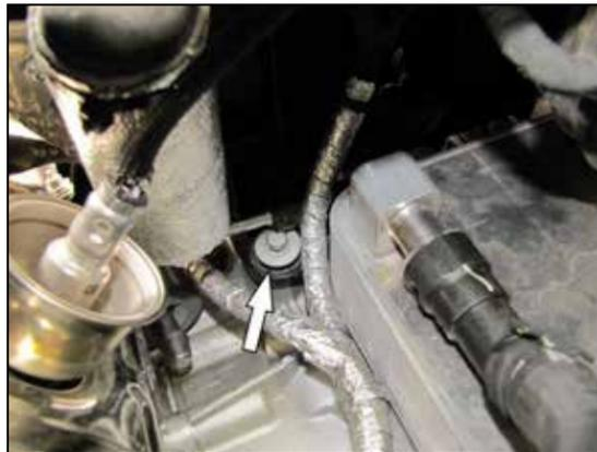
10. Remove the bolt that secures the passenger side of the air box to the transmission.
