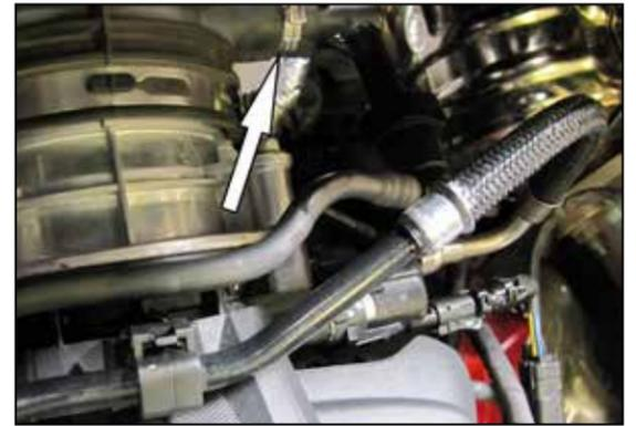
11. Cut the one time use clamp that secures the CCV hose and then disconnect the CCV hose from the factory intake tube. Loosen the hose clamp that secures the intake tube to the throttle body.
