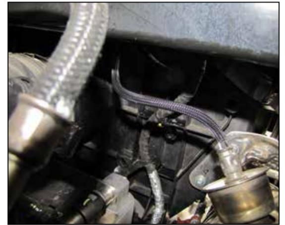
13. Disconnect the wiring harness's that attach to the rear of the air filter assembly.
