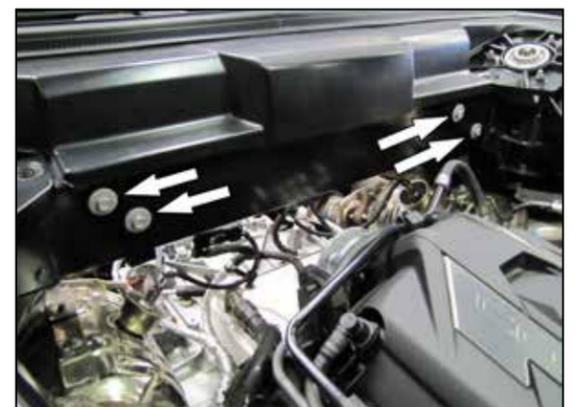
15. Install the two-heat shield mounting brackets to the chassis cross member using the four-air box mounting bolts.
