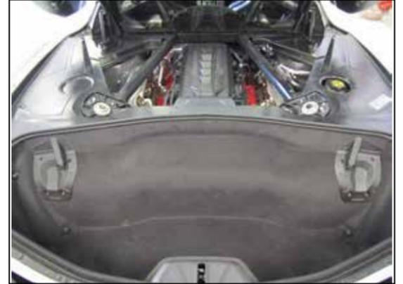
32. Reinstall the filter access panel, carpet and top stowage mounts using the factory hardware.
