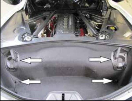
2. Open the rear hatch and locate the two roof storage mounts. Remove the bolts that secure the storage mounts and set the mounts aside. Remove the two wing nuts at the bottom of the compartment that secure the carpet.
