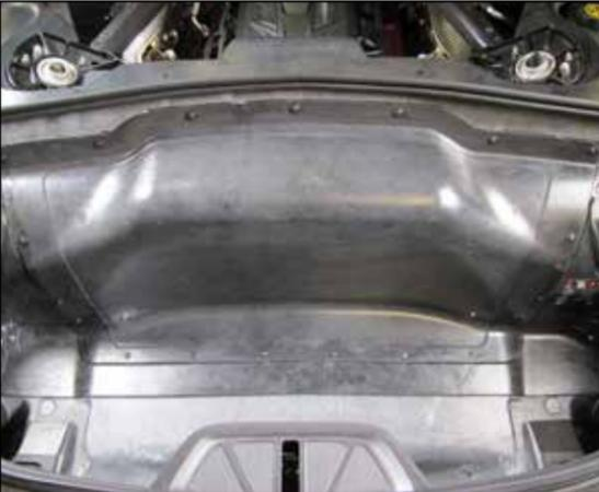
4. Remove the nineteen bolts that secure the air filter access panel and then remove the panel and set aside.
