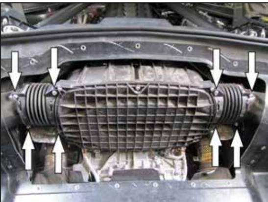
5. Remove the eight bolts that secure the two fresh air intake ducts and then remove the two ducts. These ducts will not be reused.
