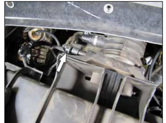
14. Pull the air filter assembly back slightly to expose "F" antenna at the top of the housing. Disconnect the electrical connection of the "F" antenna and then remove the air filter assembly from the vehicle. Remove the two fresh air duct extensions from the vehicle. These ducts will not be reused.
