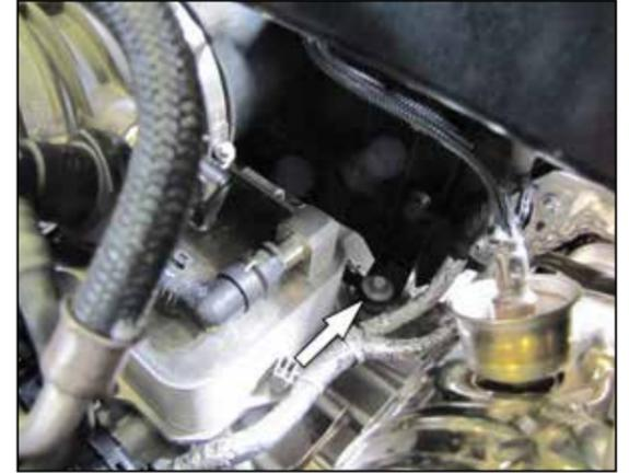
12. Remove the driver's side lower air box mounting bolt.
