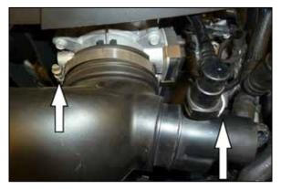
3. Loosen the hose clamp that secures the intake tube to the throttle body. Depress the locking tab and then disconnect the CCV hose from the intake tube.
