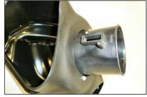
6. Install the provided mass air flow housing into the K&N air filter housing, rotate 180 degrees so the sensor will be on the top and then secure with the provided hardware.
