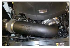
12.Install the K&N intake tube into the hump coupler and then into the coupler at the throttle body, adjust for best fit and then secure with the provided hose clamps.
