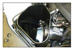
8. Install the K&N air filter housing assembly into the vehicle so the mounting studs insert into the factory grommets.
