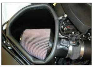
14. Install the provided edge trim onto the top of the air filter housing as shown. Some trimming of excess edge trim will be necessary.
