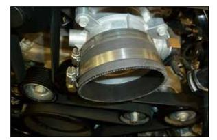
10. Install the remaining coupler onto the throttle body and secure with the provided hose clamp.
