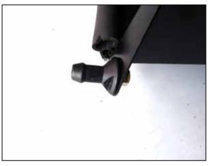
11. Attach the plastic air box mount with hardware provided to the bottom of the heatshield. Secure and tighten.
