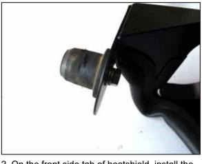
12. On the front side tab of heatshield, install the threaded boss with hardware and secure and tighten. Remove the factory rubber isolator from the OEM air box and attach to the threaded boss like image shown.
