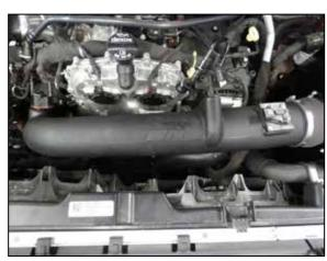
20. Install the K&N intake tube into vehicle and position. Tighten clamps.
