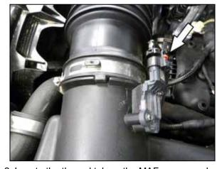
2. Locate the the red tab on the MAF sensor and slide back, Disconnect the MAF sensor harness. Pull back the MAF harness line away from air box.
