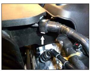
3. Depress the locking tab and disconnect the CCV.
