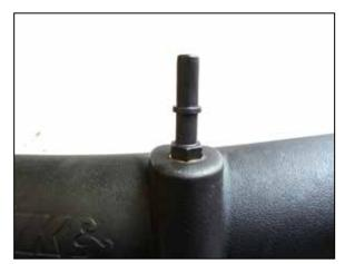
18. Install the guick connect to the threaded insert on the K&N intake tube. Secure and tighten.
