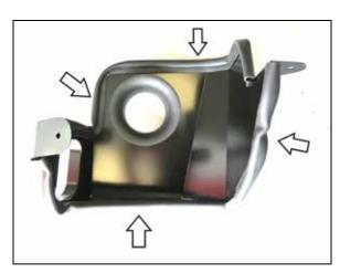
10. Install the edge trim to the top and bottom of the heatshield as shown. Cut to length like image shown using side cutters.
