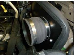
15. Install the step hose with clamps to the turbo. Install the hump hose with clamps to the filter adaptor.
