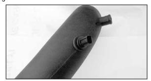
26c. Remove the air temperature sensor from the stock intake tube and install it into the grommet installed in the K&N<sup>®</sup> intake tube in the provious step as shown.
