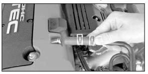
8. Remove the crank case vent hose from the vent on the cam cover.
