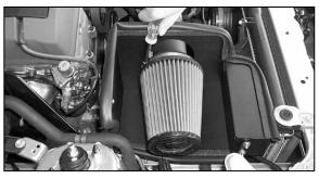
33. Install the K&N<sup>®</sup> air filter onto the K&N<sup>®</sup> intake tube and secure with the provided hose clamp. NOTE: Drycharger<sup>®</sup> air filter wrap; part number RC-5149DK is available to purchase separately. To learn more about Drycharger<sup>®</sup> filter wraps or look up color availability please visit http://www.knfilters.com<sup>®</sup>.
