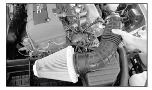
5. Loosen the hose clamp at the throttle body, then, remove the stock intake tube.
