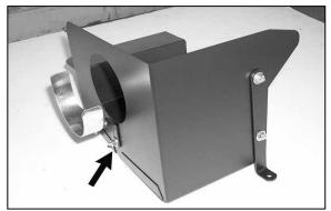
21. Using the provided hardware attach the saddle bracket assembly to the heat shield.
