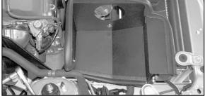
24. Using the provided hardware, install the heat shield assembly and secure the brackets to the original air box mounting locations.
