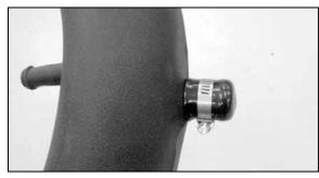
28a. On vehicles not equipped with an air injectino pump, install the provided "Caplug" onto the vent port on the K&N<sup>®</sup> intake tube and secure with the provided hose clamp as shown.
