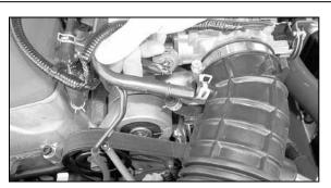
4. Remove the crank case vent hardline from the stock intake tube.
