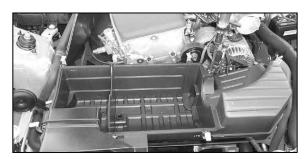
6. On vehicles equipped with air control solenoid, loosen and remove the screw and push clip that secures the air control solenoid valve to the air box base.
