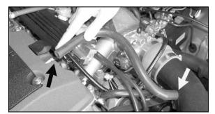
29. Attach the provided 1/2" hose to the crank case vent on the cam cover, then attach the other end to the vent on the K&N<sup>®</sup> intake tube.
