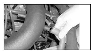
28. On vehicles equipped with air injection pump, attach the air injection hose to the fitting on the  $K\&N^{\odot}$  intake tube.
