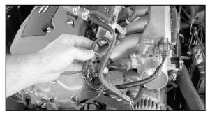
13. Remove the pipe assembly.
