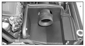
32. Install the radiused adapter onto the K&N<sup>®</sup> intake tube.
