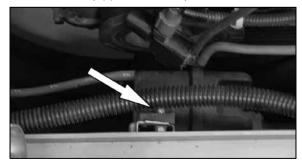
17a. Remove the bolt shown that secures the vacuum canister to the chassis.
