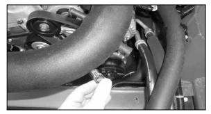
26a. On vehicles equipped with an air temperature sensor, position the air temperature sensor wiring harness on the intake tube for best fit and mark the position on the intake tube with a marker for drilling.
