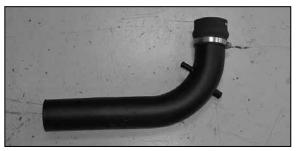
25. Install the silicone hump hose with provided hose clamps, onto the K&N<sup>®</sup> intake tube as shown.
