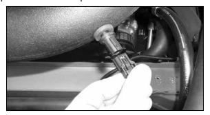
28b. On vehicles equipped with an air temperature sensor, reconnect the air temperature sensor electrical connection as shown.
