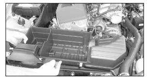
2. Release the 6 clips that retain the air box top, then remove the top.
