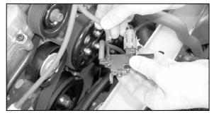
11. On vehicles equipped with air injection pump, detach the vacuum hose from the air control solenoid valve vacuum control solenoid valve.
