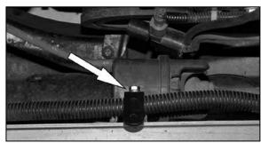
17b. Using the provided hardware, install the provided bracket (083155) along with the provided spacer and the factory vacuum canister. NOTE: The spacer should be placed between the bracket and vacuum canister.
