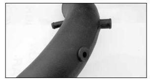
26b.On vehicles equipped with an inlet air temperature sensor, remove the intake tube from the vehicle and drill a 5/8"id hole at the spot indicated in the previous step. Install the provided grommet into the hole as shown.
