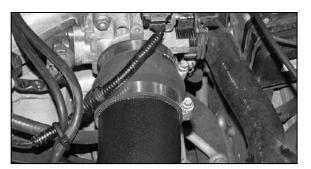
26. Install the intake K&N<sup>®</sup> tube and secure the hump hose to the throttle body as shown.
