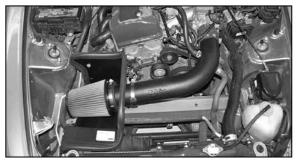
34. Reconnect the vehicle's negative battery cable. Double check to make sure everything is tight and properly positioned before starting the vehicle.
