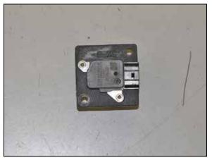
14. Install the mass air sensor into the provided adapter and secure with the provided hardware.
