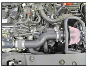
16. Install the K&N<sup>®</sup> intake tube assembly into the coupling hoses, adjust the tube for best fit and then secure with the provided hose clamps.
