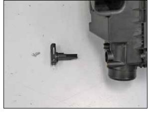
13. Remove the mass air sensor from the factory air filter housing.
