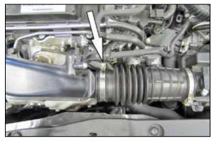
4. Loosen the hose clamp that secures the intake hose to the turbo inlet pipe and then remove the air filter housing and hose assembly. **NOTE: K&N Engineering, Inc., recommends that customers do not discard factory air intake.**
