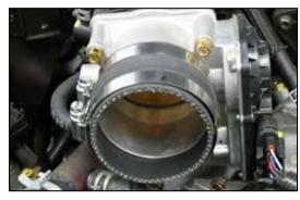
20. Install the silicone hose (08434) onto the throttle body and secure with the provided hose clamp.
