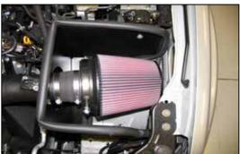
27. Install the air filter assembly onto the intake and secure with the provided hose clamp.
