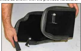
15. Install the edge trim onto the heat shield as shown.
