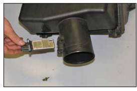
21. Remove the two screws, which secure the mass air sensor to the stock air box and then remove the mass air sensor from the air box.
