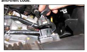
2. Disconnect the mass air sensor electrical connection and unhook the harness from the air box
