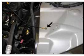
18. Remove the bolt, which secures the ground strap to the inner fender.
