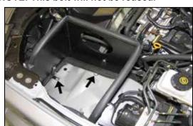
19. Install the heat shield assembly into the vehicle and secure with the provided hardware.
