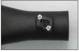
22. Install the mass air sensor into the K&N<sup>®</sup> intake tube and secure with the provided screws and spacers.
