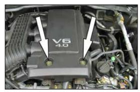
28. Reinstall the engine cover removed in step #4 and secure with the factory mounting bolts.
