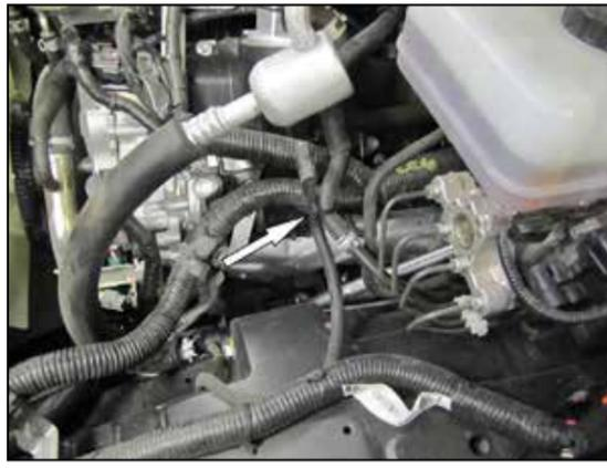
12. On 4 wheel drive models, secure the front differential vent line to the EVAP vent line.
