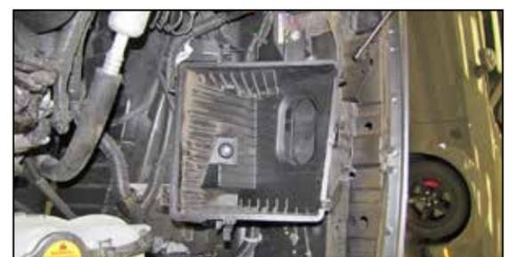
6. Remove the bolt that secures the lower air filter housing to the inner fender and then remove the lower air filter housing from the vehicle.
