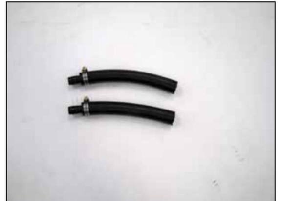
20. Install the provided union fittings into the provided vent hose and secure with the provided hose clamps.
