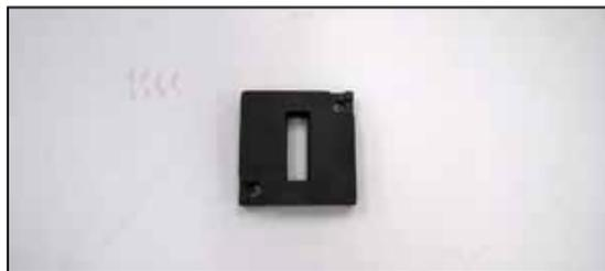
15. Install the provided gasket onto the back of the mass air sensor adapter.
