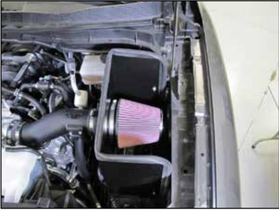
23. Install the K&N® air filter and secure with the provided hose clamp.
