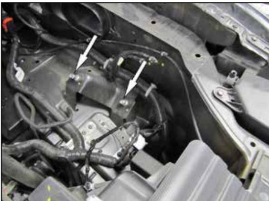
11. Remove the two-factory air filter housing mounting studs from the inner fender.
