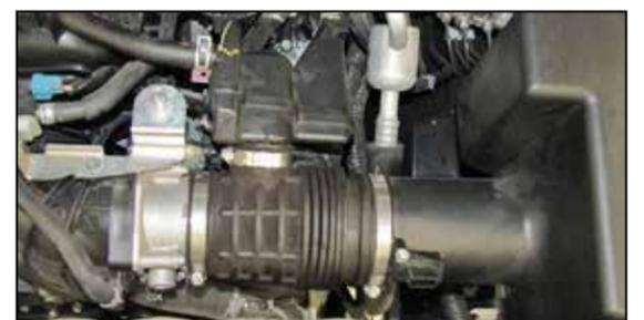
5. Loosen the hose clamp at the throttle body, unclip the upper air filter housing and disconnect the crank case vent lines from the intake tube. Remove the upper air filter housing, intake tube and factory air filter from the vehicle.
