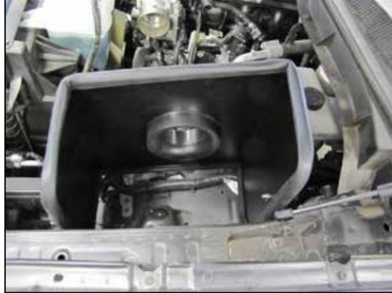
13. Install the heat shield onto the inner fender and secure with the provided hardware.
