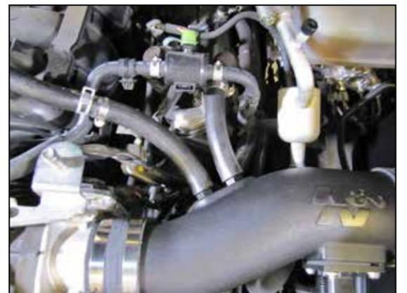
21. Install the vent fittings into the factory vent hoses and then onto the fittings installed into the K&N® intake tube.
