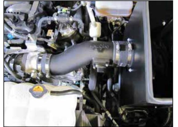
19. Install the provided coupler (08698) onto the intake tube (Do not tighten). Install the intake tube into the coupler at the throttle body and align with the filter adapter. Secure the coupler hose and intake tube with the provided hose clamps.
