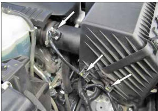
2. Disconnect the mass air sensor electrical connection and then unclip the harness from the air filter housing.
