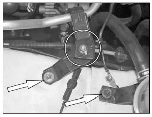
12. On vehicles equipped with the A/C mounting bracket, remove the A/C mounting bracket and loosen the nut. Then, remove the power steering reservoir mounting bolt.
