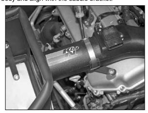
28. Secure the K&N® intake tube to the saddle bracket with the provided hose clamps also tighten the hose clamp at the the throttle body.
