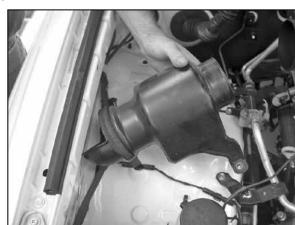
6. Remove two bolts that secure resonator to inner fender, then remove resonator from vehicle as shown.
