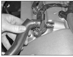
19. Remove crank case vent hose from valve cover.
