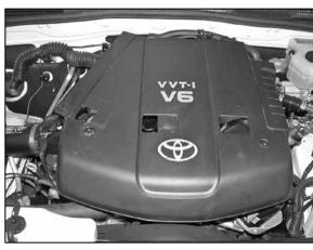
33. Re-install the engine cover using the original nuts removed in step #1.
