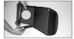
16. Install the edge trim onto the heat shield as shown. Trim if needed.
