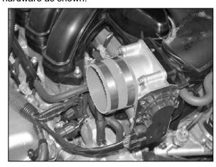
21. Install the provided silicone hose (08434) onto throttle body with the provided hose clamp as shown.
