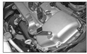
20. Install the saddle bracket assembly onto the threaded boss on the cam cover with the provided hardware as shown.
