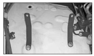
15. Mount the two provided brackets onto the vehicle with the provided hardware.
