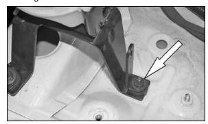
14. Remove the 12mm bolt that retains the power steering reserve to vehicle, then mount the provided bracket (07158) onto the vehicle with the bolt that was removed.
