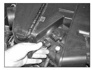
7. Disconnect the two mass air wire harnesses retaining clips from air box, then disconnect the mass air sensor electrical connection.
