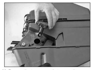
22. Remove the two screws that secure the mass air sensor to the air box assembly, then remove the mass air sensor as shown.
