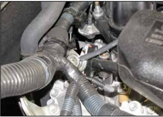
4. Unhook the fuel pressure vent line from the fuel pressure regulator.
