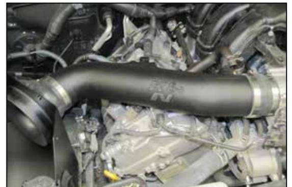
28. Install the K&N® intake tube into hump hose at the filter adapter and then into the silicone hose at the throttle body, align the tube for proper fit and then tighten the hose clamps.
