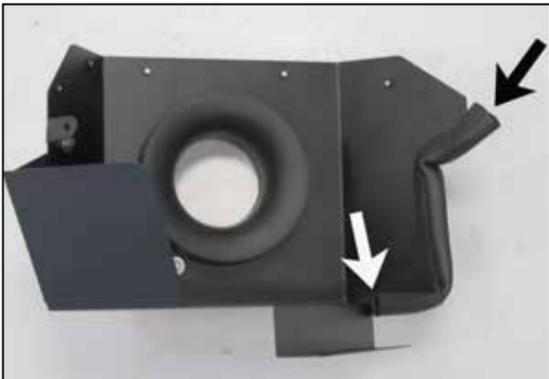
18. Install the 10.5" long piece onto the heat shield as shown.
