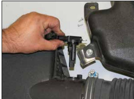
23. Remove the screws which secure the mass air sensor to the factory air box and then remove the mass air sensor from the air box.
