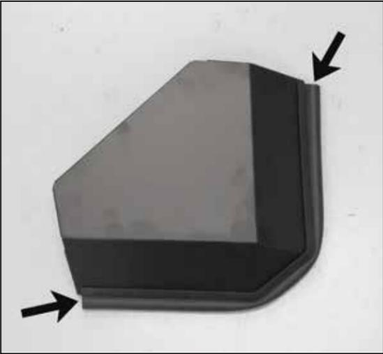
32. Install the remaining 19" piece of edge trim onto the heat shield cover as shown.
