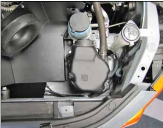
19a. Install the air injection pump onto the heat shield and forward rubber mounted stud and then secure with the provided hardware. Reconnect the air injection pump electrical connection.
