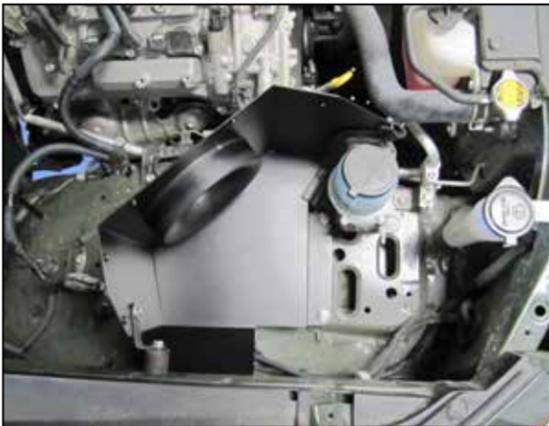
19. Set the heat shield onto the rubber mounted studs and secure with the provided hardware. **NOTE: On models that had a horn attached in this location, be sure to reattach the horn between the heat shield bracket and rubber mounted stud.**
