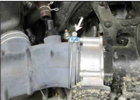
7. Loosen the hose clamp which secures the intake tube to the throttle body.
