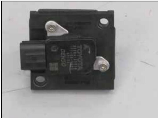
24. Install the mass air sensor into the K&N® mass air sensor adapter and secure with the provided hardware.
