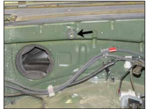
13. Install the 6mm rubber mounted stud into the inner fender location shown.
