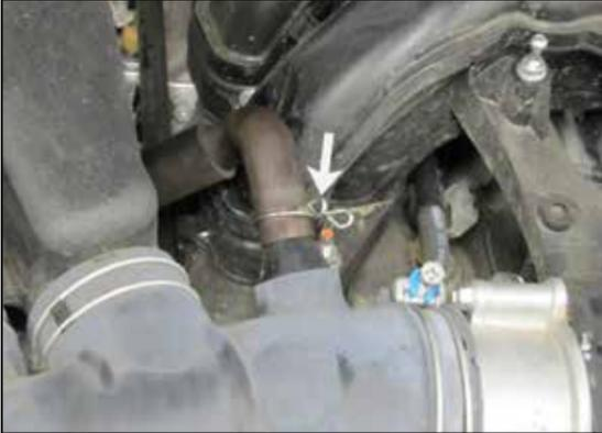
5. Disconnect the crank case vent hose from the stock intake tube.
