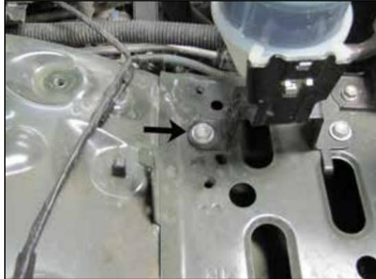
10. Remove the rear P/S reservoir mounting bolt shown.
