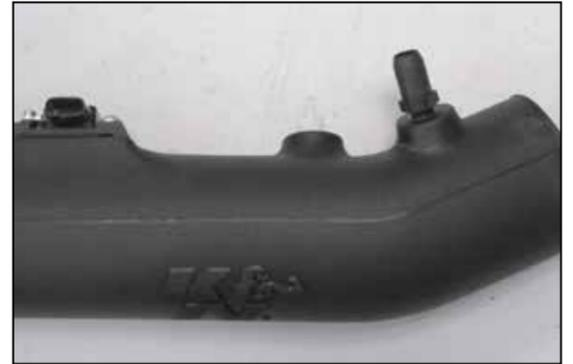
26. Install the 5/8 vent fitting into the K&N® intake tube as shown.
