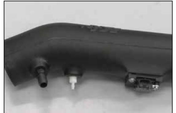
27. Install the 3/16 vent fitting into the K&N® intake tube as shown.
