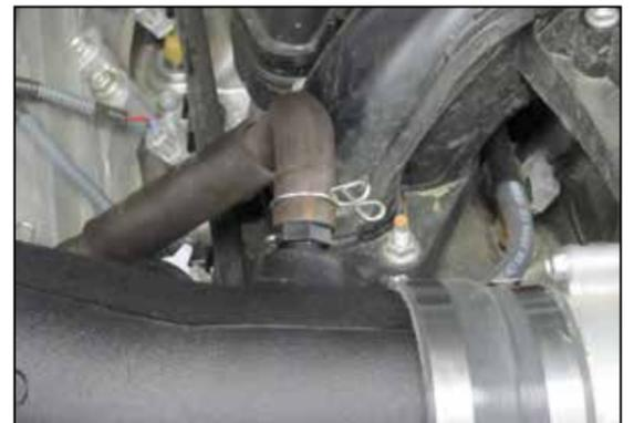
29. Connect the crank case vent line to the 5/8 vent fitting and secure with the factory spring clamp.
