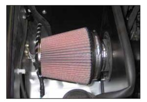
29. Install the filter assembly onto the K&N<sup>®</sup> intake tube and secure with the provided hose clamp. NOTE: Drycharger<sup>®</sup> air filter wrap; part # RF-1042DK is available to purchase separately. To learn more about Drycharger® filter wraps or look up color availability please visit http://www.knfilters.com®.
