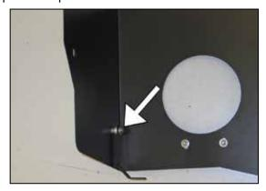
13. Install the provided heat shield mounting bracket (07190A) onto the heat shield using the provided hardware and spacer as shown.
