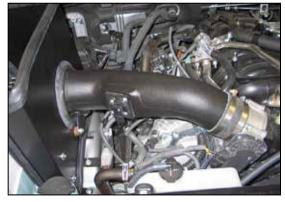
26. Install the K&N<sup>®</sup> intake tube assembly into the silicone hose at the throttle body and align with the tube mounting bracket on the heat shield. Secure the tube with the provided hardware and hose clamp.
