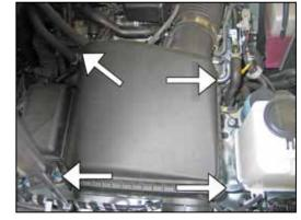
7. Release the four laches's securing the upper airbox to the lower airbox.
