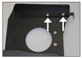
12. Install the heat shield mounting bracket (070902A) onto the heat shield as shown using the provided spacers and hardware.
