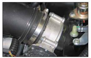
6. Loosen the hose clamp that secures the factory intake tube to the throttle body.
