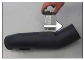
23. Install the mass air sensor assembly into the  $K\&N^{\textcircled{0}}$  intake tube as shown using the provided hardware.
