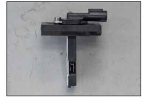
22. Install the mass air sensor into the K&N<sup>®</sup> mass air sensor adapter and secure with the provided hardware.
