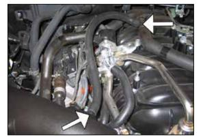
31. Install the provided crankcase vent line onto the NPT fitting installed into the K&N<sup>®</sup> intake tube and connect the open end onto the factory Tee.
