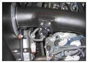
32. Reconnect the mass air sensor electrical connection.
