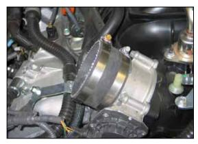
25. Install the provided silicone (08630) hose onto throttle body and secure with the provided hose clamp.
