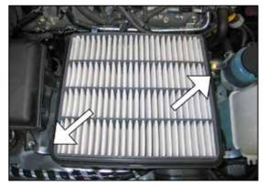
9. Loosen the two bolts securing the lower airbox into the vehicle.
