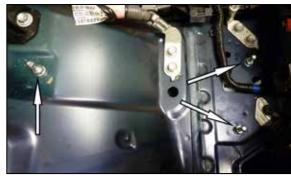
8. Remove the three air filter housing mounting studs from both the left and right sides.
