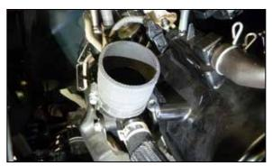
9. Install the provided couplers onto the turbo inlets and secure with the provided hose clamps.
