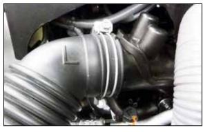
4. Loosen the hose clamps that secure the factory upper intake tubes and then remove the upper housings and intake tubes.
