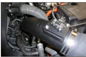
17. Install the K&N intake tubes into the couplers and adjust for best fit then secure with the provided hose clamps.
