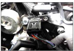
28. Using the provided bracket and hardware, mount the vacuum sensor to the engine as shown and then connect the vacuum line from the tee fitting connected to the ejector fitting.
