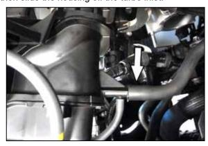
11. Disconnect the vent line shown from the manifold and remove the manifold from the vehicle.
