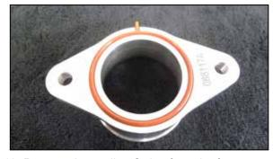
13. Remove the sealing O-ring from the factory turbo manifold and install it into the K&N turbo inlet flange.
