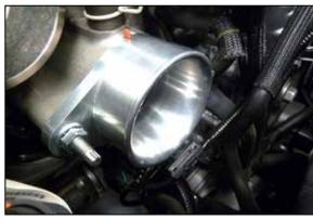
14. Install the K&N turbo inlet onto the turbo and secure with the factory mounting nuts.
