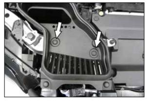
2. Push down the center of the two retaining pins to unlock them, then lift the complete fresh air duct assembly and remove it from the vehicle.
