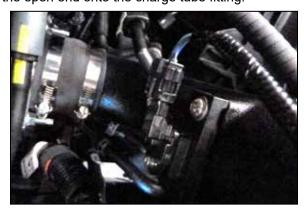
27. Reconnect the MAF sensor electrical connection.
