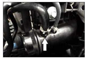
8. Release the spring clamp that secures the vent line shown to the charge tube manifold and then disconnect the hose from the manifold.
