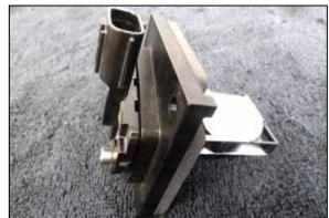
16. Install the gasket onto the K&N maf adapter. Remove the maf sensor from the factory housing and install it into the K&N adapter and secure with the provided hardware.
