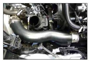
7. Release the spring clips that secure the charge tube quick connect fittings and then remove the charge tube assembly from the vehicle.
