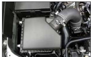
5. Disconnect the intake tube and remove the stock intake system from the vehicle.
