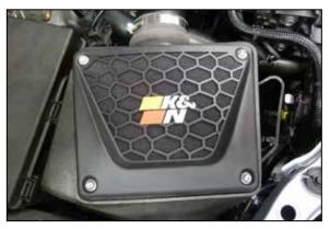
30. Assemble the pre-filter lid and install it onto the K&N air filter housing using the provided hardware.
