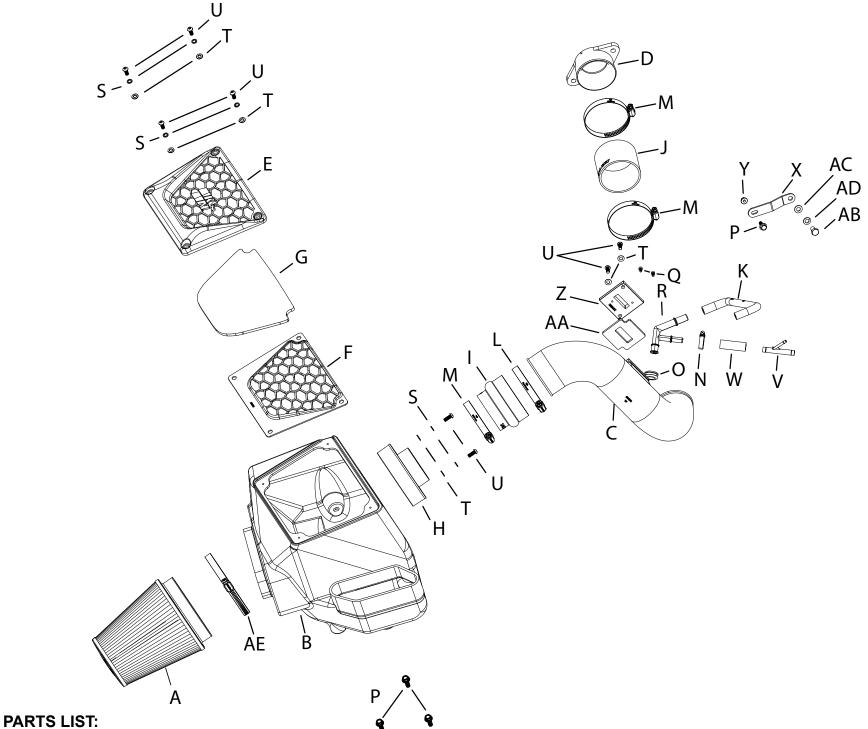
Description Part # Description Qty. Part # Description Qty. Part # Qty. AIR FILTER RU-2800 Κ HOSE; EVAP 5/16" 085196 U **BOLT**; M6 X 1 X 16MM 8 07730 087592 **AIRBOX** HOSE CLAMP; #56 08620 FITTING; VACUUM 82936 HOSE CLAMP; #48 HOSE; 3/8"ID X 2"L С TUBE 087593 08601 W 5-1002 3 D FLANGE: TURBO 088117 N HOSE CLAMP; #004 21850 BRACKET; "Z" 26545 FRAME; PRECLEANER TOP 088208 Ε O GROMMET; 9/16" KITGRMT02 Y NUT; M6, HEX, SERRATED 444.460.04 P BOLT; M6-1 X 20 4 1-2038
