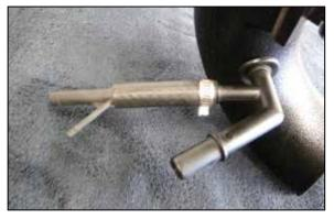
19. Install the Ejector fitting assembly into the K&N intake tube using the provided grommet.
