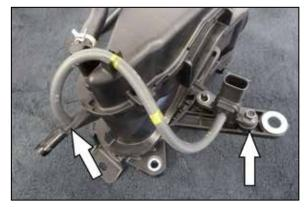
12. Disconnect the vacuum line shown, remove the sensor mounting bolt and then remove the sensor.
