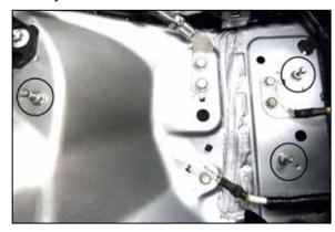
6. Remove the three air-filter housing mounting studs shown.
