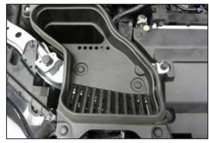
31. Reinstall the factory fresh air duct and secure with the factory pins.
