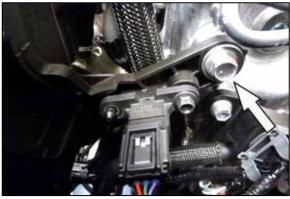
9. Remove the solenoid mounting bolt and disconnect the vacuum switch electrical connection.
