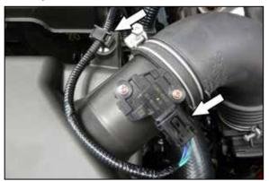
3. Disconnect the mass air sensor electrical connection and unhook the wiring harness from the retaining clip.
