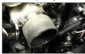
15. Install the provided coupler onto the turbo inlet and secure with the provided hose clamp.
