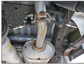
5. Remove muffler assembly from remaining hangers.
