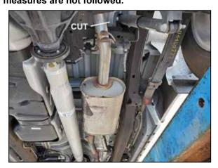
2. Unless a vehicle lift is available cutting the stock exhaust will be mandatory to remove. Cut rear tailpipe 2" from rear hanger just above the axle where shown.
