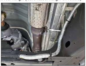
4. Once rear tail pipe has been removed loosen front conical clamp connecting tail pipe to head pipe.
