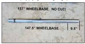
8. For vehicles with 147.5" wheelbase 9.5" must be cut off the end opposite to the conical end connecting to the head pipe (As shown). For vehicles with 157" wheelbase it does not need to be cut.
