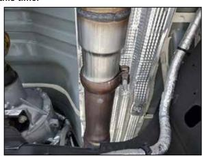
11. Slide mid pipe and muffler assembly into position on the vehicle by first using the hangers on the muffler end. Once inserted, then slide assembly rearward allowing the mid pipe to move into position to seat against head pipe with the factory conical clamp.
