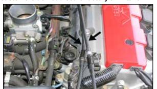
13. Secure the throttle cable and cruise control cable (if equipped) to the stock clips as shown.
