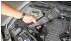
5. Remove the air inlet duct.
