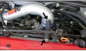
20. Install the provided silicone hose onto the crankcase vent on the cam cover, then connect the other end to the vent on the K&N® intake tube as shown.
