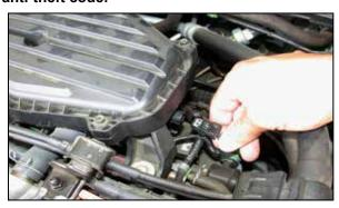
2. Disconnect the air temperature sensor electrical connection as shown.
