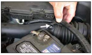
3. Unclip the battery cable from the air inlet duct as shown.
