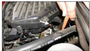
8. Loosen the hose clamp that secures the plenum to the throttle body as shown.
