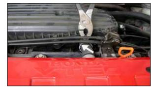
9. Using a pair of pliers, depress and pull back the hose clamp on the crankcase vent at the cam cover.
