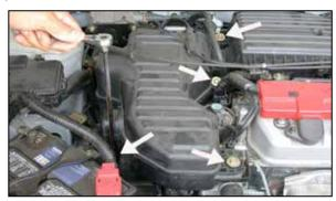
6. Loosen and remove the four bolts that secure the air intake resonator.
