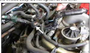
15. Install the rubber mounted stud onto the stock resonator mounting location as shown.
