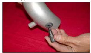
17. Install the provided rubber grommet into the hole on the K&N® intake tube, then install the air temperature sensor into the grommet as shown. NOTE: Before installing the grommet and air temperature sensor, Inspect the inside of the tube for any debris, then clean the inside out with water and a towel. Inspect the tube one more time before proceeding to the next step.
