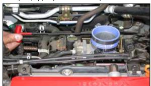
14. Install the silicone hose and hose clamps onto the throttle body. Do not tighten at this time.
