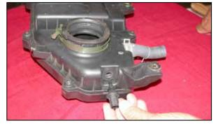
16. Remove the air temperature sensor from the throttle body plenum as shown.
