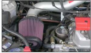
22. Install the K&N® air filter onto the K&N® intake tube and secure with the provided hose clamp. Adjust for best fit and clearance then tighten all hardware.
