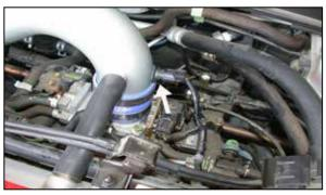
21. Reconnect the air temperature sensor electrical connection as shown.
