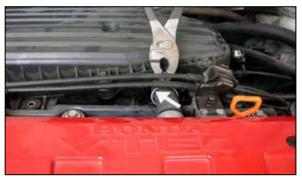
9. Using a pair of pliers, depress and pull back the hose clamp on the crankcase vent at the cam cover.
