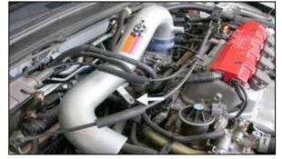
18. Install the K&N<sup>®</sup> intake tube onto the throttle body, then, line up the bracket with the rubber mounted stud as shown. Tighten hose clamps at this time.
