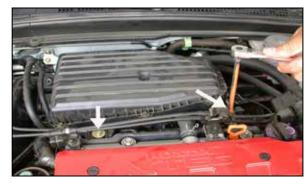
7. Loosen and remove the two bolts that secure the throttle body plenum.
