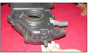
16. Remove the air temperature sensor from the throttle body plenum as shown.
