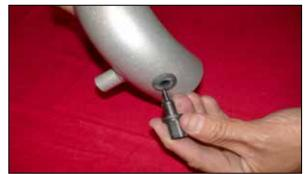
17. Install the provided rubber grommet into the hole on the K&N<sup>®</sup> intake tube, then install the air temperature sensor into the grommet as shown. NOTE: Before installing the grommet and air temperature sensor, Inspect the inside of the tube for any debris, then clean the inside out with water and a towel. Inspect the tube one more time before proceeding to the next step.
