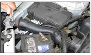
4. Loosen and remove the two bolts that secure the air inlet duct as shown.
