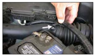
3. Unclip the battery cable from the air inlet duct as shown.
