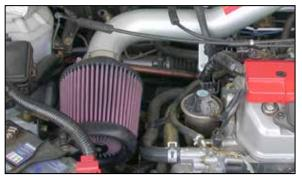
22. Install the K&N<sup>®</sup> air filter onto the K&N<sup>®</sup> intake tube and secure with the provided hose clamp. Adjust for best fit and clearance then tighten all hardware.
