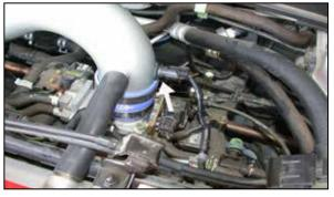
21. Reconnect the air temperature sensor electrical connection as shown.
