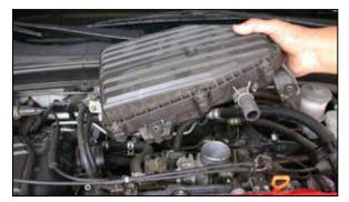
10. Pull firmly upwards to remove the throttle body plenum as shown.
