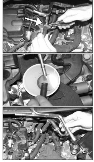
11. Using pliers, remove the coolant hose from the thermostat housing and the throttle body adaptor (a small amount of coolant may drain, have a cup ready to catch the fluid).
