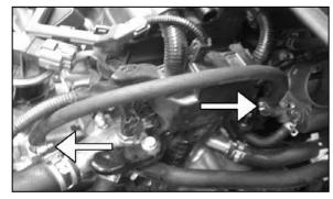
12. Install the provided coolant hose and secure with provided hose clamps.
