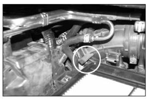
8. Using the 5.5mm socket and short extension, loosen the hose clamps that secure the factory intake tube to the throttle body.
