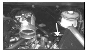
17. Install the K&N<sup>®</sup> intake tube into the vehicle. Attach the bracket to the threaded hole from the factory airbox mounting point. Tighten hose clamps at the throttle body.
