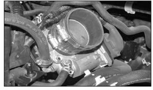
13. Install the silicone hose and hose clamps onto the throttle body as shown.
