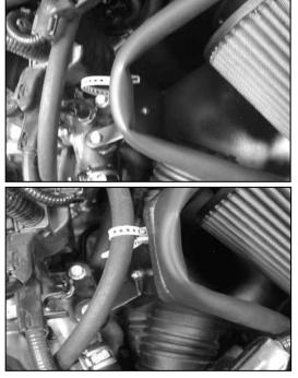
29. Install cable tie to the heat shield, then secure to the hose as shown.
