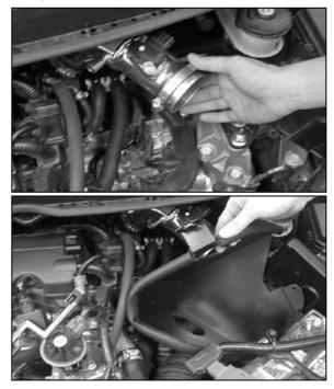
23. Slide the provided hose clamp onto the K&N<sup>®</sup> intake tube, then install the heat shield. **NOTE: On automatic transmission equipped vehicles, it will be necessary to remove the air filter and heat shield from the vehicle to check the transmission fluid level.**
