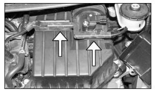
3. Press the two tabs that hold the MAF sensor wire harness to the factory airbox and unclip.
