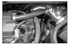
27. Attach the provided CCV-hose with #8 hose clamps, from the engine valve cover to the K&N<sup>®</sup> intake tube as shown.
