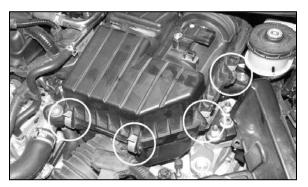
4. Unclip the four clips that secure the upper airbox in place, then remove the upper factory airbox.
