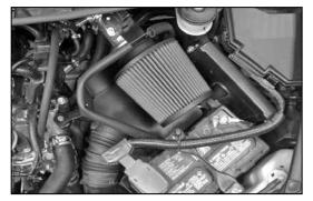
26. Install the air filter onto the K&N<sup>®</sup> intake tube.
