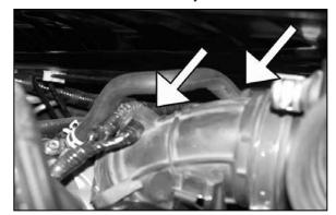
9. Unclip the EVAP canister hose and two wire
