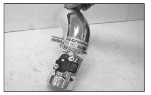
15. Secure the MAF sensor to the K&N<sup>®</sup> intake tube with the provided hardware.
