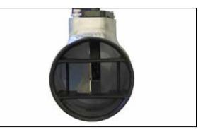
15a. Install the provided venturi into the end of the intake tube as shown.
