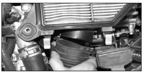
7. Remove the air inlet hose from the lower factory airbox.
