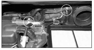
5. Unclip the two clips that secure the CCV-hose (one is located on the engine's valve cover, the other is located on the lower factory airbox) and disconnect the CCV-hose
