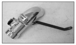
16. Attach the "Z" bracket to the K&N<sup>®</sup> intake tube using the provided hardware.
