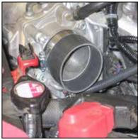
22. Install silicone hose (#08440) onto the throttle body and secure with the provided hose clamp.
