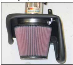
21. Install the K&N  $^{\hbox{\scriptsize I}{\sc B}}$  air filter onto the air filter adapter and secure with the provided hose clamp.
