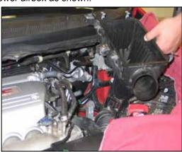
8. Remove the complete lower airbox assembly from the vehicle as shown.
