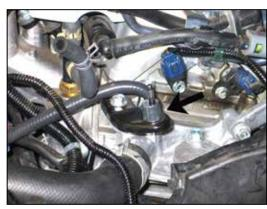
23. Install the provided spacer onto the airbox mounting stud as shown.
