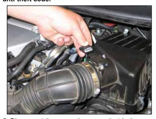
2. Disconnect the mass air sensor electrical connection. Un-clip the mass air sensor wiring harness from the upper airbox.
