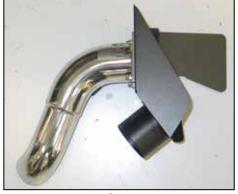
18. Install the K&N<sup>®</sup> intake tube onto the exposed studs and secure with the provided hardware.
