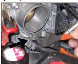
11. Release the spring clamp that secures the coolant bypass hose to the throttle body, then disconnect the coolant bypass hose from the throttle body. Remove the bypass/crank case vent hose assembly from the vehicle.
