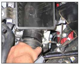
7. Un-hook the fresh air supply duct from the lower airbox as shown.
