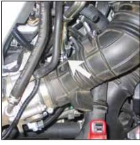
4. Release the crankcase breather hose spring clamp. Release the hose clamp that secures the intake tube to the throttle body.
