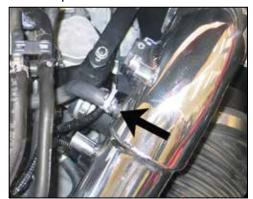
26. Install the EVAP hose onto the  $K\&N^{\textcircled{R}}$  intake tube and secure it with the factory hose clamp.
