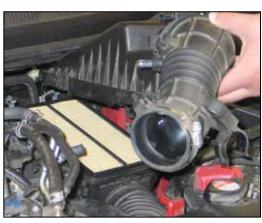
5. Release the six upper airbox clips, then remove the upper airbox and intake tube assembly as shown.
