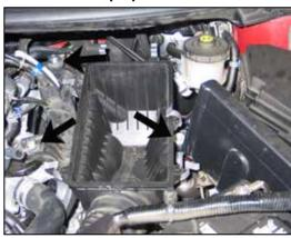
6. Remove the one nut and two bolts that secure the lower airbox to the vehicle.
