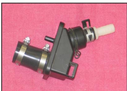
25. Insert the hose mender into the crank case vent chamber. Secure using the stock clamp removed in step # 3.
