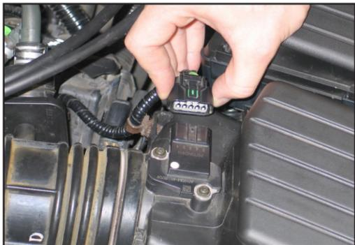
2. Depress the locking tab and remove the mass air sensor connector. Remove the clips securing the mass air sensor harness to the stock airbox and intake tube.
