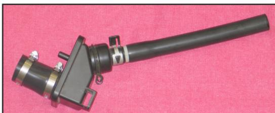
26. Install the provided silicone hose onto the hose mender as shown.
