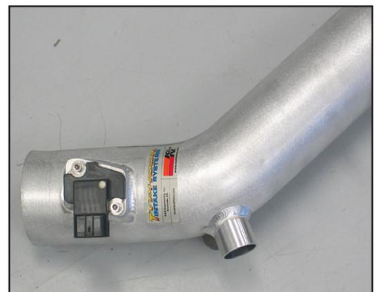
21. Install the mass air sensor into the K&N® intake tube with the provided hardware as shown.
