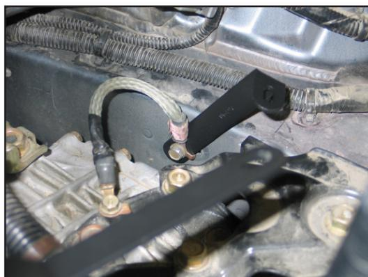
15. Install angled "L" bracket (#06497) onto the frame rail. Secure the "L" bracket and ground strap using the bolt removed in step #14.
