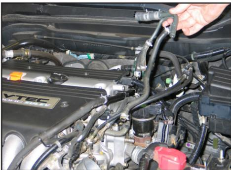
10. Remove the stock coolant hose assembly from the vehicle.
