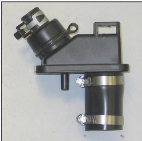
23. Install the provided silicone hose (#084074) onto the stock crankcase vent chamber. Secure with the provided hose clamps as shown.
