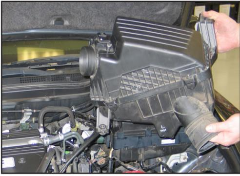
7. Unclip the wiring harness from the bottom of the stock airbox and remove from the vehicle.
