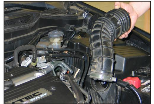
5. Pull firmly to remove the stock intake tube from the airbox. Remove the intake tube from the vehicle.
