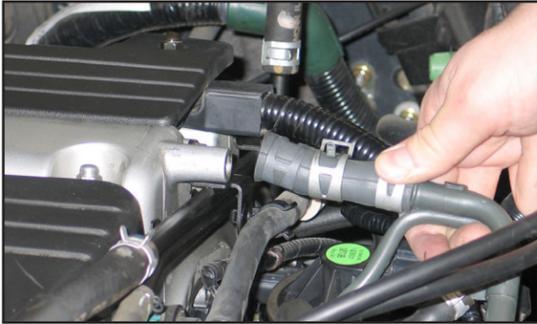
8. Depress the spring clamp and remove the crankcase vent hose from the valve cover.
