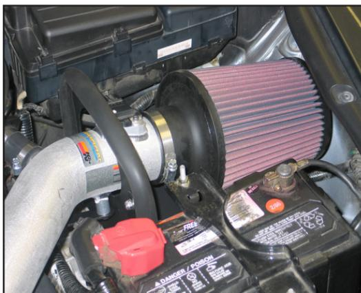
29. Install the K&N® air filter onto the intake tube as shown.
