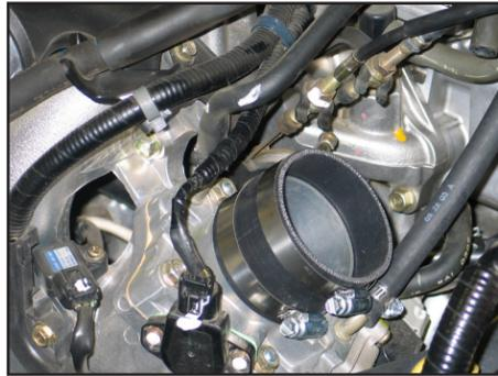
12. Install the provided silicone hose (#08440) onto the throttle body. Secure with the provided hose clamp as shown.
