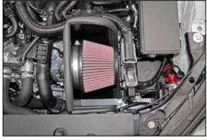
9. Flex the heat shield inward and install the K&N<sup>®</sup> air filter onto the filter adapter and secure with the provided hose clamp.
