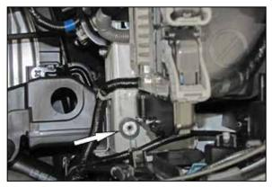
7. Thread the provided rubber mounted stud into the factory air filter housing location shown.
