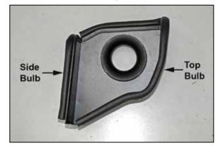
6. Install the provided side bulb and top bulb edge trim onto the heat shield as shown. NOTE: Some trimming of the edge trim will be necessary.
