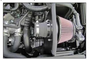
10. Install the provided coupler (08713) onto the filter adapter and secure with the provided hose clamp.
