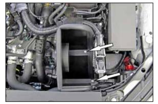
8. Install the heat shield assembly into the vehicle and secure with the provided hardware to the rubber mounted stud and the rear factory air filter housing mounting location.
