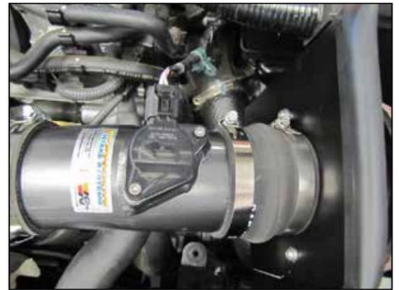
16. Reconnect the mass air sensor electrical connection.
