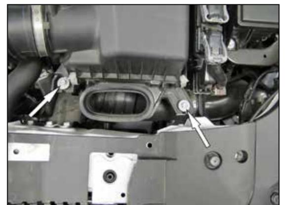
5. Remove the two bolts that secure the air filter housing to the inner fender and then remove the bolts from the vehicle.
