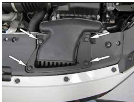
4. Remove the four push pins that secure the fresh air intake duct and then lift the fresh air intake duct out to remove it from the vehicle.
