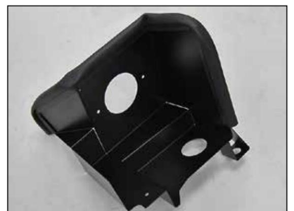
6. Install the provided edge trim onto the heat shield as shown.
