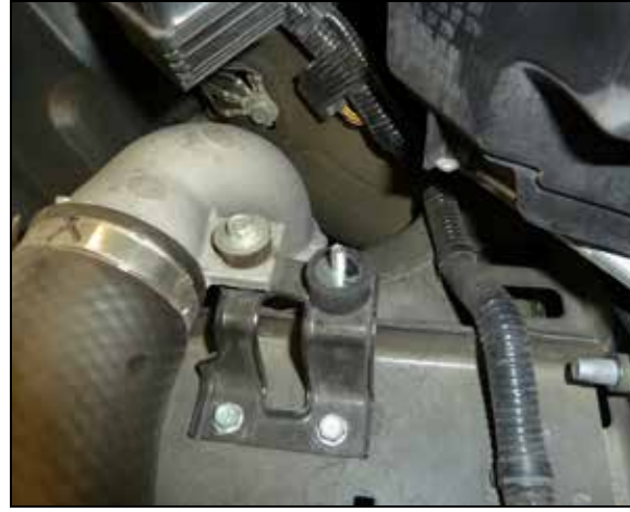
9. Install the provided rubber mounted stud onto the factory filter housing bracket as shown.
