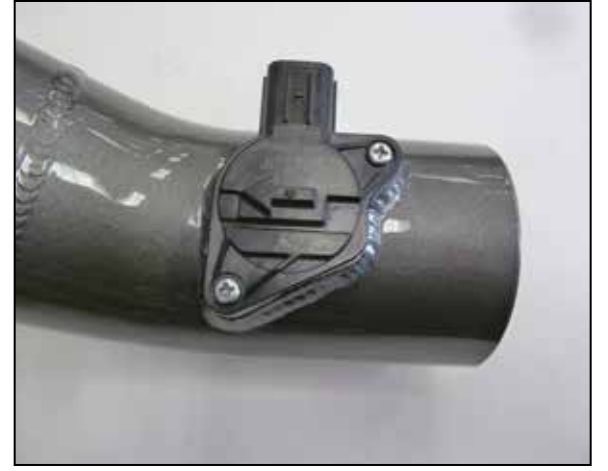
13. Remove the mass air sensor from the factory housing and install it into the K&N intake tube and secure with the factory mounting bolts.
