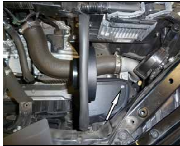
10. Install the heat shield into the vehicle and secure with the provided hardware.
