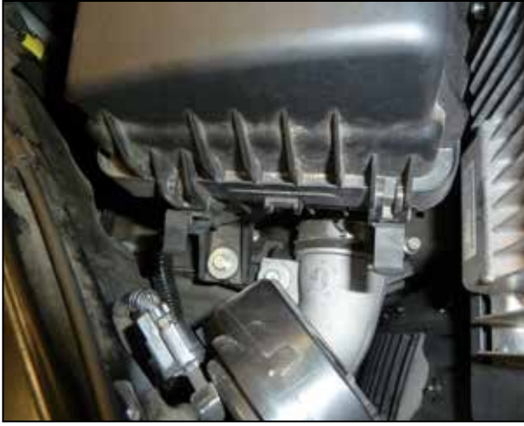
5. Release the two spring clamps that secure the air filter housing lid, remove the lid, intake hose and factory air filter.
