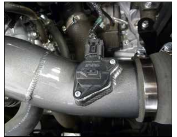
15. Reconnect the mass air sensor electrical connection.
