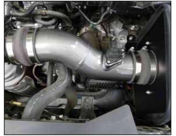
14. Install the K&N intake tube into the couplers, adjust for best fit and then secure with the provided hose clamps.
