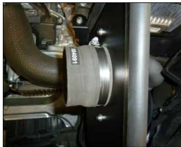
11. Install the provided step coupler onto the filter adapter and secure with the provided hose clamp.
