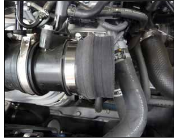
12. Install the provided hump coupler onto the turbo inlet manifold and secure with the provided hose clamp.
