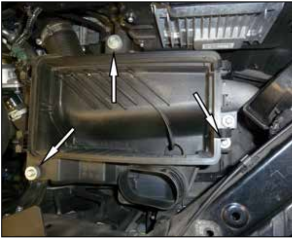
6. Loosen the three bolts that secure the lower air filter housing to the inner fender and then remove the housing from the vehicle.
