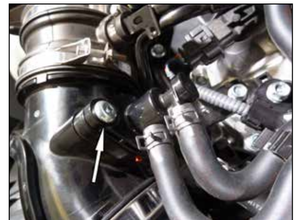
3. Remove the two bolts that secure the EVAP fitting to the factory intake tube and remove the fitting from the intake tube.
