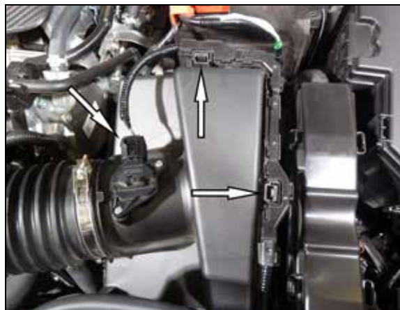
2. Disconnect the mass air sensor electrical connection and then unhook the wiring harness from air filter housing.
