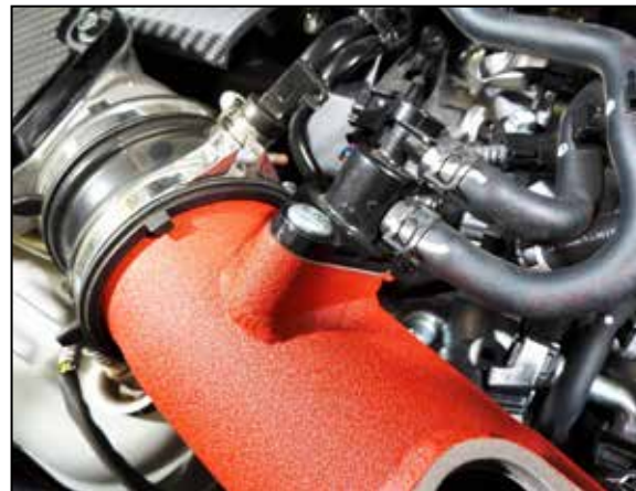
15. Install the EVAP fitting into the K&N intake tube and secure with the factory hardware.
