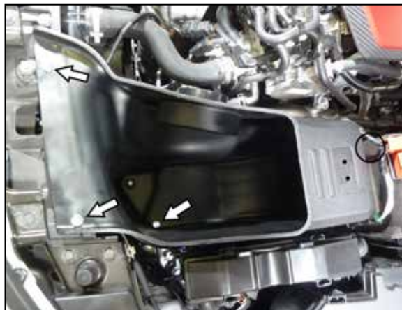
9. Set the K&N air filter housing into the vehicle, secure the rear of the housing with the factory mounting bolt. Secure the front of the housing with the hardware provided.
