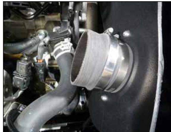
12. Install the provided hump hose onto the filter adapter and secure with the provided hose clamp.
