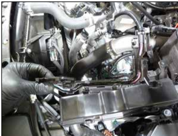
7. Remove the hard plastic cover from the mass air sensor harness pig tail.
