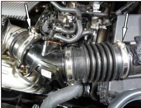
4. Loosen the two hose clamps shown and then remove the factory intake tube assembly.
