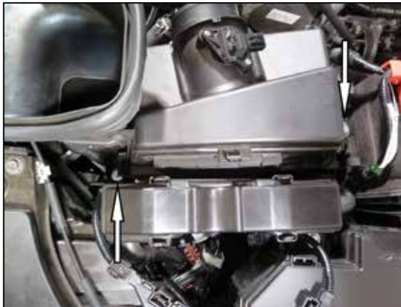
6. Remove the two bolts that secure the air filter housing and then remove the housing from the vehicle.
