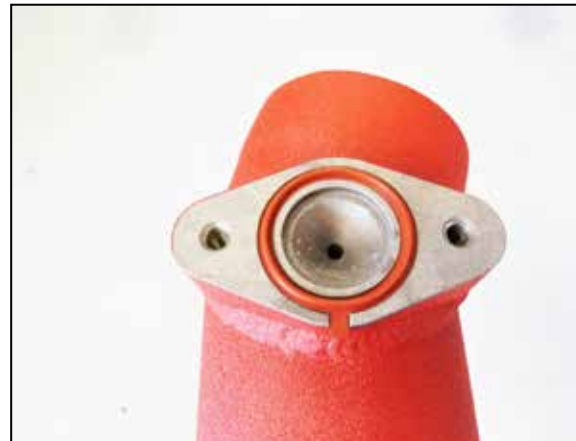
13. Remove the EVAP fitting O-Ring from the factory intake system and install it into the K&N intake tube as shown.
