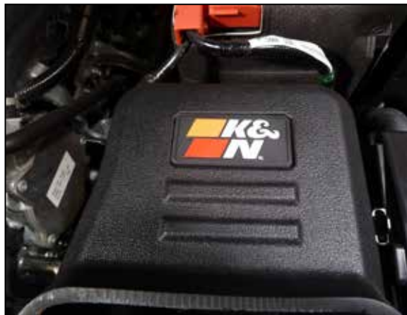
10. Snap the K&N badge into the filter housing.
