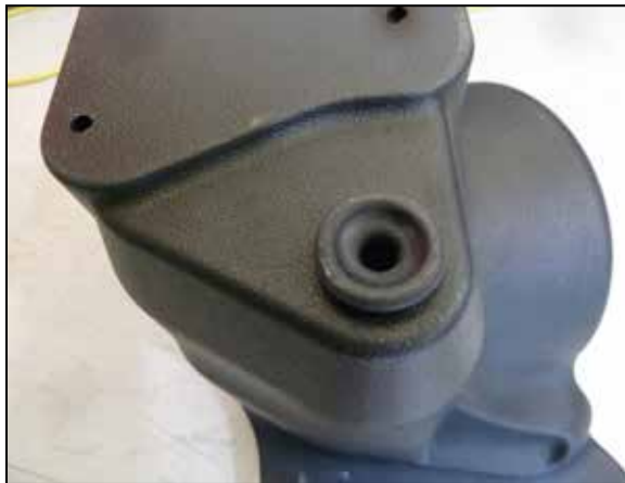
8. Remove a mounting grommet from the factory air filter housing and install it into the K&N filter housing as shown.
