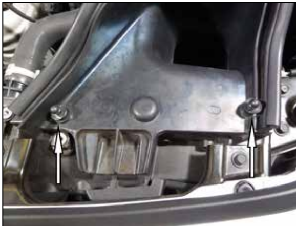
5. Remove the two bolts that secure the fresh air duct to the core support.
