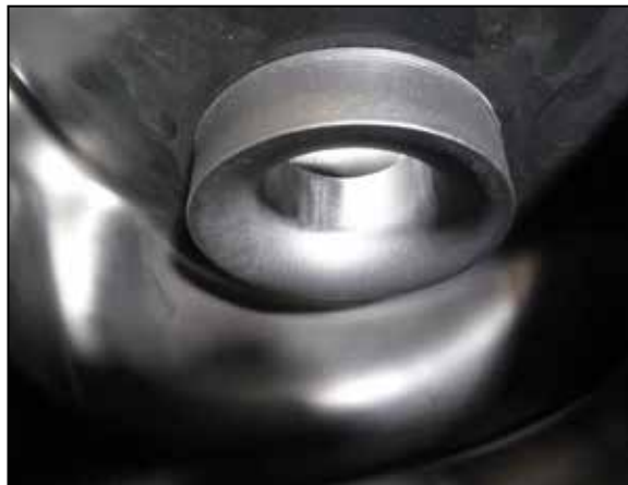
11. Install the provided filter adapter into the K&N filter housing and secure with the provided hardware.
