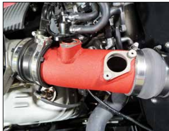
14. Install the K&N intake tube into the hump coupler and factory coupler, adjust for best fit and secure with the factory and provided hose clamps.
