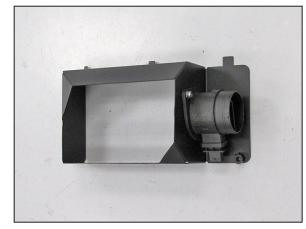
8. Remove the O-ring from the mass air sensor and then secure the mass air sensor to the provided heat shield using the hardware provided.
