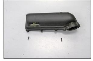
10. Remove two of the factory air filter housing screws from the upper air box.
