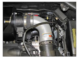
13. Install the K&N<sup>®</sup> intake tube into the factory intake hose and then into the hose at the mass air sensor. Secure the intake tube with the factory and provided hose clamp
