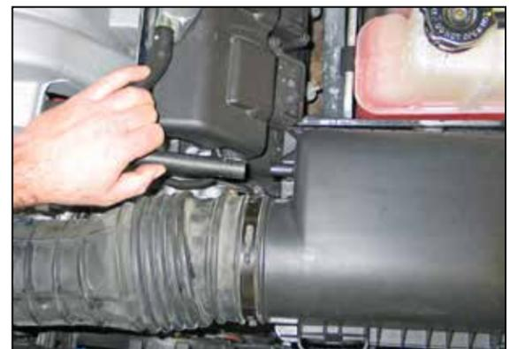
6. On SRT-8; 6.1L vehicles, disconnect the crankcase vent hose from the airbox as shown.
