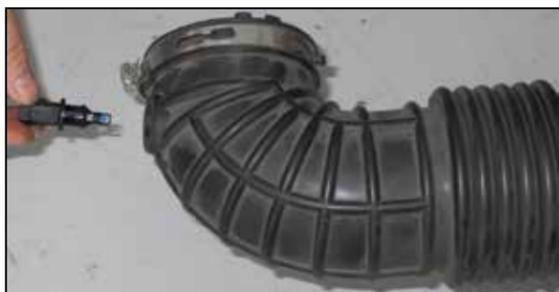
15. Remove the inlet air temperature sensor from the stock intake hose as shown.
