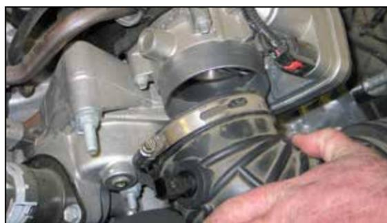
4. Loosen the hose clamp that secures the intake tube to the throttle body and pull the intake tube off of the throttle body.
