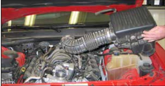
8. Lift and remove the complete intake assembly from the vehicle.
