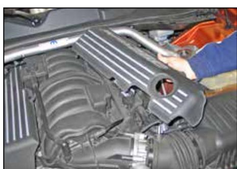
3. Lift up and remove the driver side ignition coil cover as shown.
