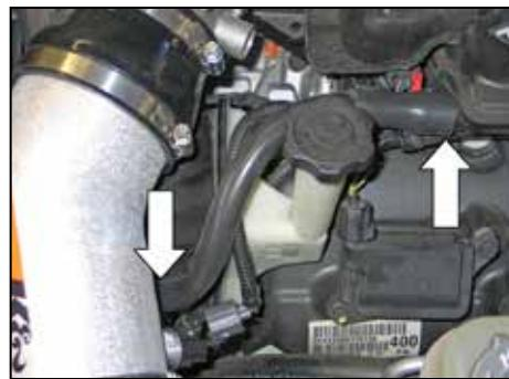
21. Attach the assembled vent hose onto the fitting installed in the K&N® intake tube; attach the open end of the vent hose to the valve cover port.
