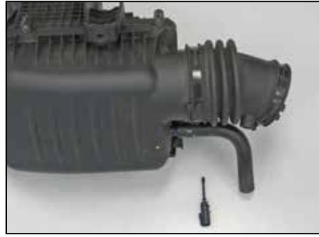
16. Remove the inlet air temperature sensor from the factory intake tube as shown.
