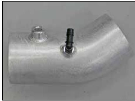
15. Install the provided 90° vent fitting into the K&N® intake tube as shown.
