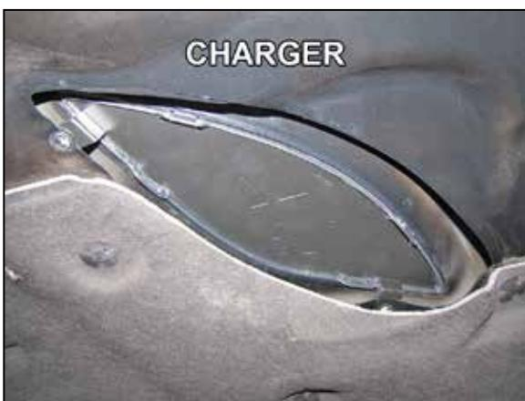
26. Install the guard so the mounting tabs are between the hood and the factory grid as shown.
