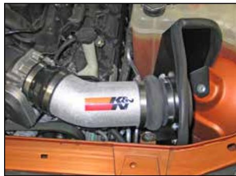
18. Install the K&N® intake tube into the silicone hump hose and then into the into the silicone step hose at the throttle body. Align the intake tube and heat shield for proper fit and then secure the intake tube with the provided hose clamps and heat shield bracket with the factory air box retaining bolt removed in an earlier step.
