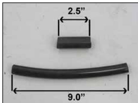
19. Cut the provided  $\frac{1}{2}$ " silicone vent hose to a length of 9" long. Also cut the 5/8" vent line to a length of 2.5" long.
