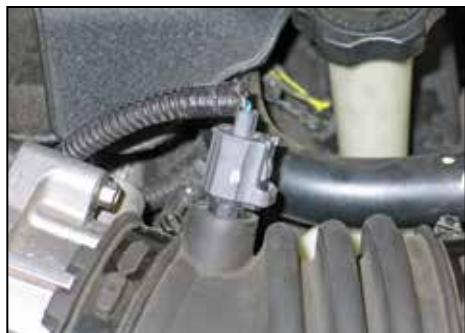
2. Disconnect the inlet air temperature air sensor electrical connection.
