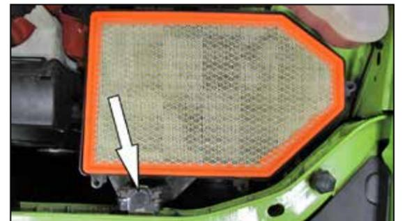
6. Remove the bolt securing the lower air filter housing to the core support and then remove the air filter housing from the vehicle.
