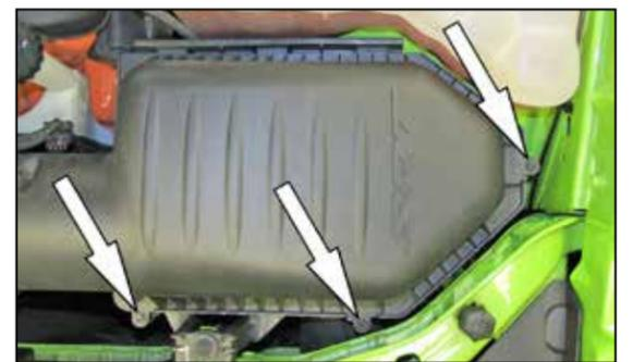
5. Loosen the three screws securing the upper air filter housing and then remove the upper air filter housing and intake tube.
