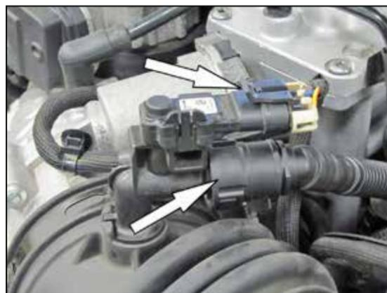
3. Disconnect the pressure sensor electrical connection and disconnect the crank case vent hose from the fitting.
