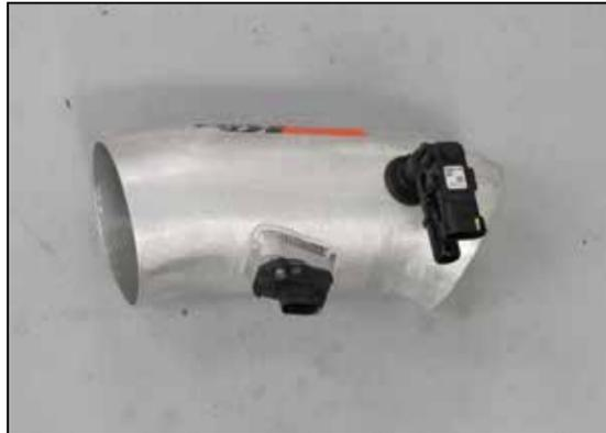
14. Install the provided grommet and pressure sensor/vent assembly into the K&N® intake tube as shown.
