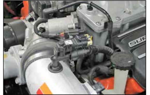
17. Reconnect the crank case vent hose and pressure sensor electrical connection.
