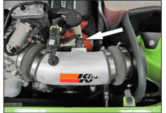
18. Reconnect the mass air sensor electrical connection.
