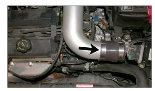
17. Install the silicone step hose and hose clamps onto the intake tube as shown.
