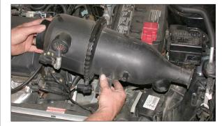
8. Pull firmly upwards to remove the air cleaner assembly as shown.
