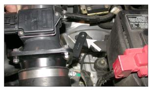
19. Slide the mass air sensor assembly into the silicone step hose, then, line up the bracket with the hole located on the battery tray as shown.
