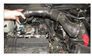
6. Loosen the hose clamp at the throttle body and at the mass air sensor, then, remove the stock intake tube as shown.
