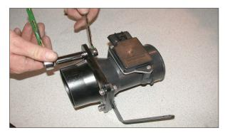
18. Assemble the stock mass air sensor, gasket, mass air adapter, and bracket using the provided hardware as shown.
