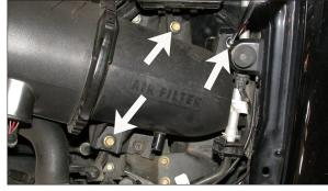
7. Loosen and remove the three bolts that secure the air cleaner assembly as shown.
