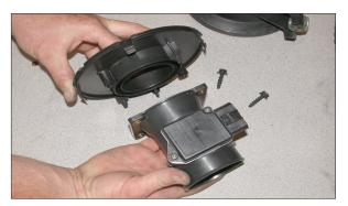
11. Remove the two bolts that secure the mass air sensor, then, remove the mass air sensor as shown.
