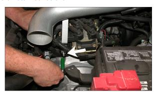
15. Secure the bracket to the stud using the provided washer and hex nut as shown.
