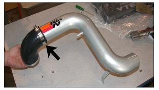
12. Assemble the 90 degree silicone hose and hose clamps onto the intake tube as shown. Due to hood clearance problems, the long end of the silicone hose should be clamped onto the tube. NOTE: Before installing the silicone hose, inspect the inside of the tube for any debris, then clean the inside out with water and a towel. Inspect the tube one more time before proceeding to the next step.
