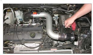
21. Tighten all hose clamps and hardware and adjust for best fit.
