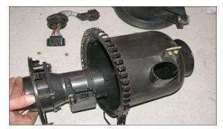
10. Remove the mass air sensor base plate from the air cleaner housing as shown.
