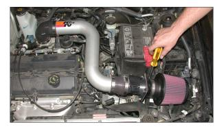
22. Install the air filter and secure with the provided hose clamp as shown.
