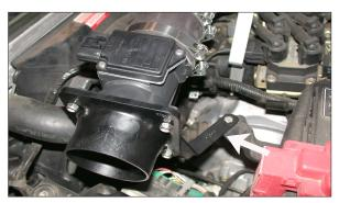
20. Secure the bracket to the battery tray using the provided hardware as shown.
