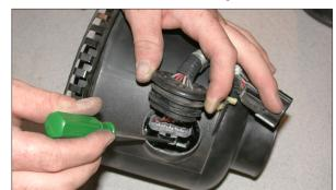
9. Pull the rubber boot back then depress the release tab to disconnect the mass air sensor electrical connection as shown.
