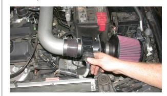
23. Reconnect the secondary and primary mass air electrical connections as shown.
