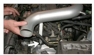
14. Line up the bracket on the tube with the stud on the water neck as shown.
