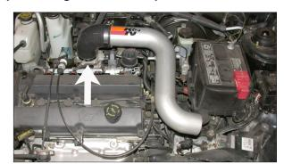
13. Slide the intake tube assembly onto the throttle body as shown, but do not tighten completely at this time.
