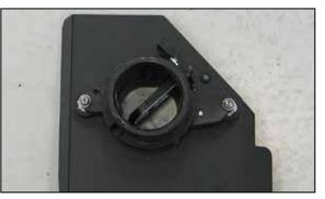
22. Secure the mass air sensor housing to the rubber mounted studs on the heat shield as shown using the provided hardware.
