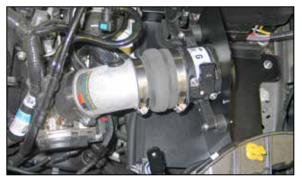
27. Install the K&N<sup>®</sup> intake tube into the silicone hose on the throttle body, then align the heat shield and secure with the provided hardware. Align the intake tube and secure with the provided hose clamps.
