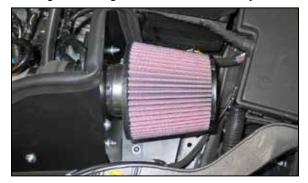
36. Install the K&N<sup>®</sup> air filter and secure with the provided hose clamp.
