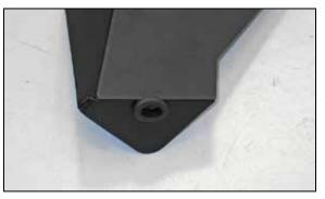
33. Install the provided 7/8"OD grommet into the  $K\&N^{\otimes}$  fresh air plate as shown.
