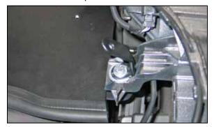
18. Using the provided hardware, secure the provided bracket (083161) to the fresh air intake scoop mount and the rubber mounted stud on the heat shield base.
