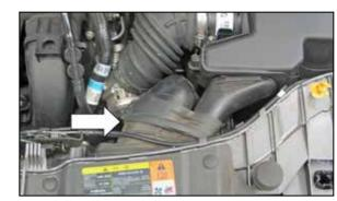
7. Release the rubber strap securing the fresh air intake scoop to the duct.
