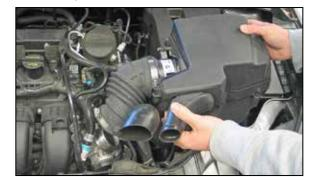
2. Release the red locking tab and then disconnect the mass air sensor electrical connection. Also unhook the mass air sensor wiring harness clip from the mass air sensor.
