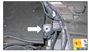
17. Place the provided fender washer onto the fresh air intake scoop mount as shown.
