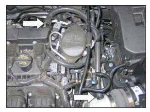
28. Install the provided silicone vent hose onto the 90° vent fitting in the K&N<sup>®</sup> intake tube and attach the open end to the valve cover port as shown.
