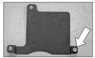
13. Install the provided rubber mounted stud onto the heat shield as shown using the provided hardware.
