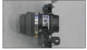
23. Install the provided hump hose (08421) onto the mass air sensor as shown and secure with the provided hose clamp.
