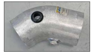
24. Install the provided 1.0"OD grommet into the K&N $^{\odot}$  intake tube as shown.
