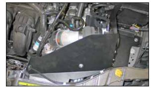
34. Pass the hood release cable through the grommet installed into the K&N<sup>®</sup> fresh air plate and then secure the fresh air plate to the heat shield and mounting bracket with the provided hardware. Reinstall the hood release cable to the hood latch.
