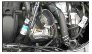
11. Install the provided silicone hose (084016) onto the throttle body and secure with the provided hose clamp.
