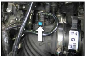
3. Depress the blue locking tab and then disconnect the EVAP vent line.
