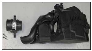
21. Remove the two bolts securing the mass air sensor housing to the air box; separate the mass air housing from the air box.
