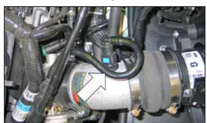
30. Install the EVAP fitting into the intake tube and then connect the EVAP vent line.
