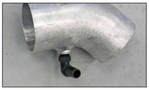
25. Install the 90° vent fitting into the K&N $^{\mbox{\tiny \$}}$  intake tube as shown.
