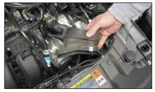
9. Remove the rubber fresh air duct from the vehicle.
