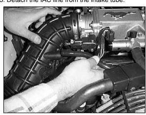
6. Detach the PCV line from the intake tube.
