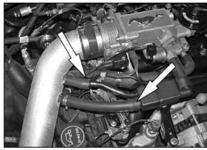
23. Reconnect the vent hoses to the K&N® intake tube as shown and tighten hose clamps.
