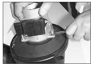
9. Loosen and remove the 4 nuts that retain the mass air sensor.
