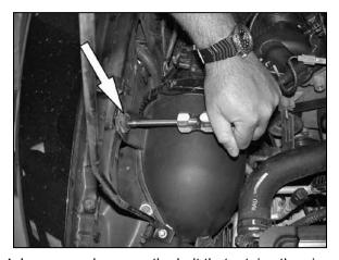
4. Loosen and remove the bolt that retains the air cleaner.
