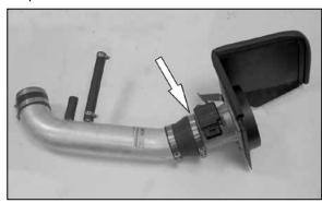
19. Install the K&N® intake tube onto the mass air sensor and snug the hose clamps, but do not tighten completely at this time.
