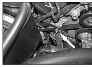
22. Slide the brackets onto the stud from step 11 and secure with the factory nut.
