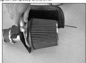
20. Install the K&N® air filter onto the filter adapter and secure with the provided hose clamp as shown.
