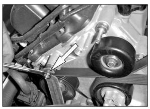
11. Loosen and remove the nut from the protruding stud on the engine.
