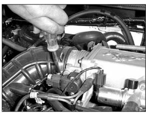
3. Loosen the hose clamp on the intake tube at the throttle body.
