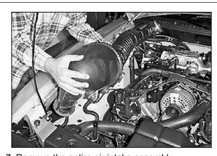
7. Remove the entire air intake assembly.
