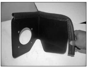
12. Install the trim seal onto the heat shield. NOTE: Some cutting and trimming will be necessary to achieve best fit.
