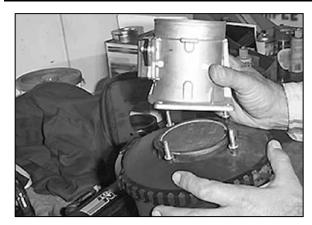
10. Remove the mass air sensor from the air cleaner.
