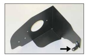
7. Install the small bracket (070812) onto the heat shield as shown and secure with the provided hardware.
