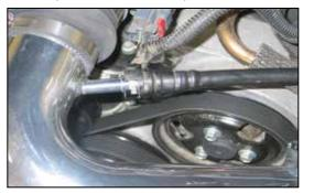
20. Connect the crank case vent hose to the K&N<sup>®</sup> intake tube as shown.
