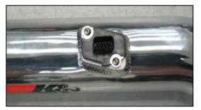
18. Install the mass air sensor into the K&N<sup>®</sup> intake tube and secure with the provided hardware.
