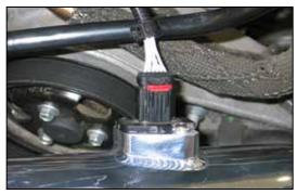
22. Install the K&N<sup>®</sup> mass air sensor harness extension into the factory wiring harness and then connect the open end into the mass air sensor.
