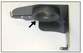
9. Secure the K&N<sup>®</sup> filter adapter to the heat shield as shown using the provided hardware.
