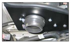
16. Install the provided step hose (084093) onto the filter adapter and secure with the provided hose clamp.
