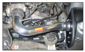
19. Install the K&N<sup>®</sup> intake tube into the silicone hose on the filter adapter and then into the silicone hose at the throttle body. Secure the intake tube with the provided hose clamps.
