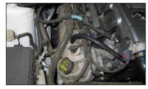
23. Connect the crankcase vent hose to the vent port on the valve cover.
