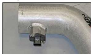
17. Install the mass air sensor into the  $K\&N^{\mbox{\scriptsize @}}$  intake tube and secure with the provided hardware.
