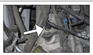
4. Release the locking tab and then disconnect the crankcase vent tube from the valve cover.
