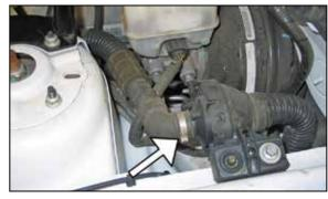
8. Cut the hose clamp securing the engine pulse hose to the engine pulse drum.
