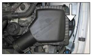
6. Remove the bolt shown that secures the factory airbox to the fender well.
