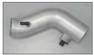
18. Install the 90° vent fitting into the K&N® intake tube as shown.
