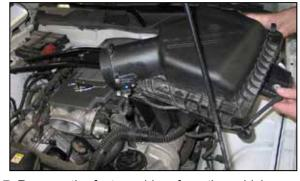
7. Remove the factory airbox from the vehicle. NOTE: K&N Engineering, Inc., recommends that customers do not discard factory air intake.
