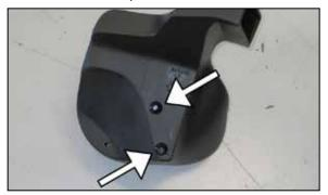
12. Install the two provided mounting studs onto the bottom of the K&N<sup>®</sup> airbox using the provided hardware.
