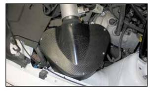
25. Install the airbox lid onto the airbox and secure with the provided hardware.
