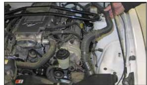
9. Remove the engine pulse hose from the vehicle.
