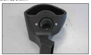
11. Install the filter adapter into the K&N® airbox and secure with the provided hardware.
