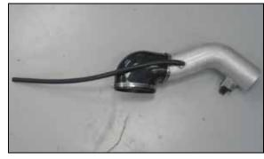
21. Install the provided crankcase vent hose onto the 90° fitting installed into the K&N® intake tube.
