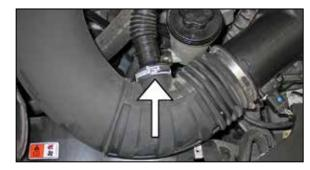
3. Release the spring clamp that secures the engine pulse hose to the factory intake tube, and then disconnect the engine pulse hose from the intake tube.
