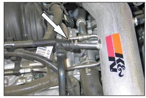
20. Connect the crankcase vent hose to the quick connect fitting on the  $K\&N^{\otimes}$  intake tube.
