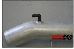
16. Install the provided 90° NPT vent fitting into the K&N $^{\mbox{\tiny ®}}$  intake tube as shown.
