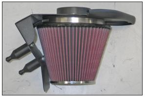
12. Install the K&N<sup>®</sup> air filter onto the filter adapter and secure with the provided hose clamp. NOTE: Drycharger<sup>®</sup> air filter wrap; part # RF-1048DK is available to purchase separately. To learn more about Drycharger<sup>®</sup> filter wraps or look up color availability please visit http://www.knfilters.com<sup>®</sup>.
