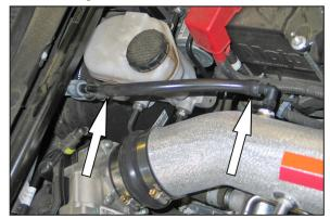
21. Connect the provided EVAP hose onto the  $90^{\circ}$  vent fitting installed in the K&N<sup>®</sup> intake tube, then connect the open end to the EVAP check valve as shown.
