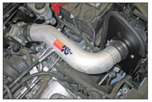
19. Install the K&N<sup>®</sup> intake tube assembly into the hose at the throttle body and then onto the filter adapter and secure with the provided hose clamp.
