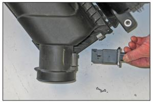
14. Remove the mass air sensor mounting bolts, then remove the mass air sensor from the factory airbox.
