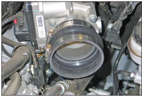
17. Install the provided silicone hose (084079) onto the throttle body and secure with the provided hose clamp.
