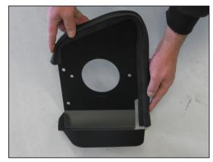
9. Install the provided edge trim onto the heat shield as shown. **NOTE: Trimming of the edge trim will be**
