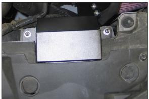
13. Install the heat shield/filter assembly into the vehicle so that the mounts snap into the factory airbox mounts.
