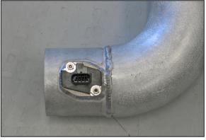
15. Install the mass air sensor into the K&N<sup>®</sup> intake tube and secure with the provided hardware.
