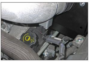
22. Reconnect the mass air sensor electrical connection.
