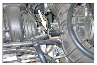
4. Release the grey locking tab and then disconnect the crankcase vent line from the intake tube.
