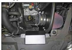
14. Install the provided fresh air scoop onto the core support and then secure the scoop to the core support and heat shield with the provided hardware
