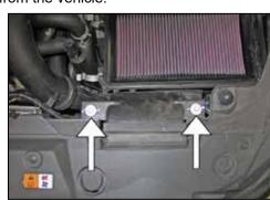
6. Remove the two bolts shown that secure the fresh air duct.
