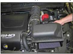
5. Remove the upper airbox/intake tube assembly from the vehicle.
