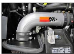
18. Install the K&N® intake tube into the silicone hump hose and then into the filter adapter's silicone hose. Secure the intake tube with the provided hose clamps.
