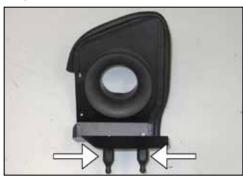
11. Install the two provided mounting studs onto the heat shield and secure with the provided hardware.
