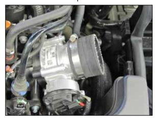
13. Install the provided silicone hose (08440) onto the throttle body and secure with the provided hose clamps.
