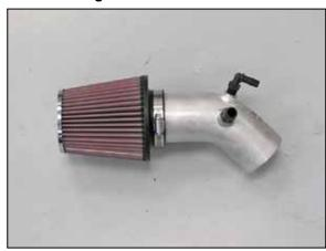
16. Install the K&N<sup>®</sup> air filter onto the K&N<sup>®</sup> intake tube and secure with the provided hose clamp.
