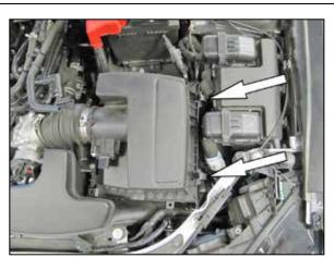
5. Release the two upper housing clips and then remove the upper housing, intake hose and air filter from the vehicle.
