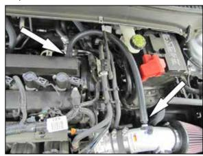
18. Install the provided crankcase vent hose onto the valve cover port and then onto the fitting installed into the K&N® intake tube as shown.
