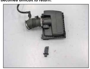
11. Remove the two screws securing the mass air sensor into the upper air box housing and then remove the sensor from the housing.
