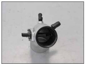
15. Install the venturi into the K&N® intake tube as shown.
