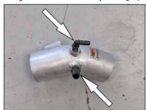
10. Install the two provided vent fittings into the  $K\&N^{\text{@}}$  intake tube as shown.
