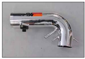
19. Install the mass air sensor into the  $K\&N^{\otimes}$  intake tube and secure with the provided hardware.
