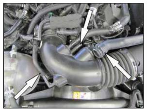
4. Depress the locking tabs and then disconnect the crank case vent hose and the EVAP vent hose. Then release the spring clamp and disconnect the sound tube from the intake tube. **NOTE: Some vehicles are not equipped with the**
