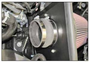
16. Install the provided hump coupler (08699) onto the filter adapter and secure with the provided hose clamp. 21. Connect the crank case vent, EVAP vent and idle by pass lines to the quick disconnect fittings installed into the K&N<sup>®</sup> intake tube. **NOTE: On vehicles not equipped with an EVAP**
