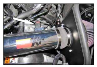
22. Connect the provided mass air sensor extension harness into the factory mass air sensor connection and then connect the other end to the mass air sensor.
