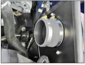
12. Install the provided coupler hose (08496) onto the filter adapter and secure with the provided hose clamp.
