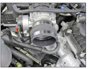
11. Install the provided hump coupler (5-323) onto the throttle body and secure with the provided hose clamp.
