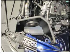
9. Install the heat shield onto the lower bracket installed in step #5 and secure with the provided hardware. Do not secure the upper bracket at this time.
