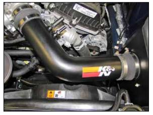
14. Install the K&N<sup>®</sup> intake tube into the coupling hoses and adjust for best fit, then secure the intake tube with the provided hose clamps.
