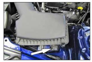
4. Remove the bolt which secures the air filter housing to the inner fender and then remove the air filter housing from the vehicle.
