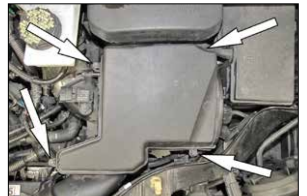
5. Loosen the four screws that secure the air filter housing lid and then remove the lid and factory air filter.
