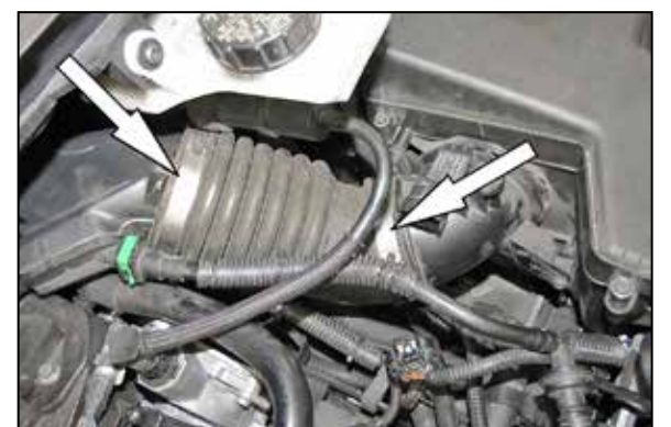
6. Loosen the two hose clamps that secure the factory intake hose.
