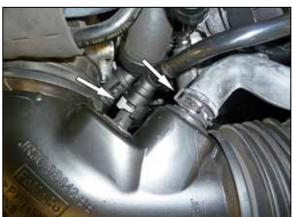
5. Disconnect the vent lines and sound tube attached to the intake tube. Loosen the hose clamps that secure the intake tube to the air filter housing and throttle body and then remove the intake tube from the vehicle.
