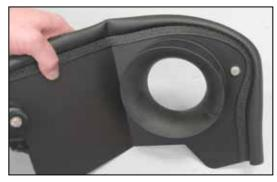
15. Apply one of the supplied gaskets to the filter adapter studs and then pass the studs through holes in the heat shield to install the filter adapter as shown.
