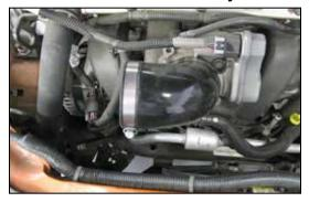
9. Install the silicone hose (084087) onto the throttle body as shown and secure with the provided hose clamp.
