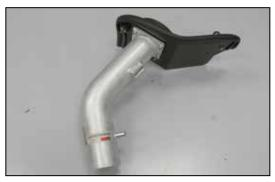
16. Install the K&N<sup>®</sup> intake tube to the filter adapter studs with the remaining gasket and then secure with the provided hardware.
