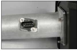
18. Install the mass air sensor into the K&N<sup>®</sup> intake tube and secure wit the provided bolts.
