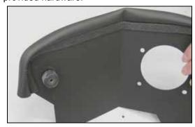
13. Install the remaining rubber mounted stud onto the heat shield as shown and secure with the provided hardware.
