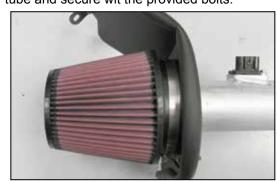
19. Install the K&N® filter onto the filter adapter and secure with the provided hose clamp.
