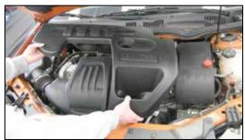
2. Remove the engine oil cap and then lift the engine cover to dislodge it from the mounting grommets and then remove the engine cover assembly.
