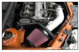
21.Install the K&N® intake tube into the silicone hose at the throttle body and align the "L" bracket with the inner airbox mounting stud as shown.
