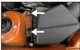
7. Remove the two nuts which secure the airbox to the inner fender.
