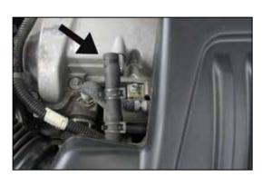
6. Using pliers loosen the clamp which secures the crankcase vent hose to the valve cover vent port and then disconnect the crankcase vent hose as shown.
