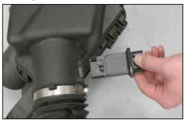
17. Remove the two screws that secure the mass air sensor and then remove the mass air sensor from the stock intake tube as shown.
