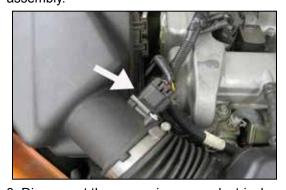
3. Disconnect the mass air sensor electrical connection.
