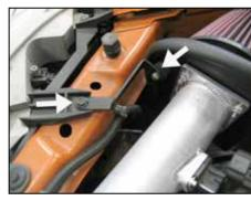
23. Install the "Z" bracket onto the headlight mounting bracket and rubber mounted stud as shown. Secure with the factory bolt removed in step #22 and the provided hardware.
