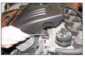
4. Using a small screw driver, release the plenum locking clip by prying the center of the plenum locking clip.
