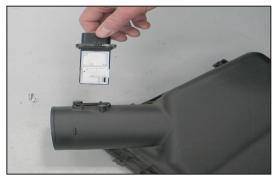
13. Remove the two mass air sensor retaining screws and then remove the mass air sensor from the air box as shown.
