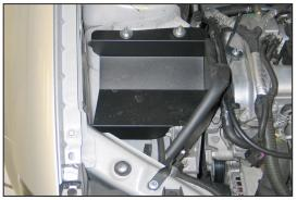
19. Set the heat shield into position on the air box mounting studs. Secure the mounting bracket to the core support with the provided hardware. Secure the heat shield to the mounting studs with the factory nuts removed in step #5.
