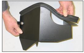
18. Install the provided edge trim onto the heat shield. Some trimming of the edge trim will be necessary.
