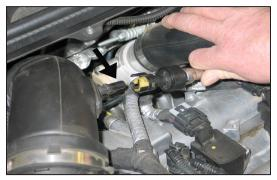
3. Release the locking tab and then disconnect the crank case vent hose from the stock intake tube.
