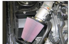
11. Install the two provided spacers onto the air box mounting studs as shown.
