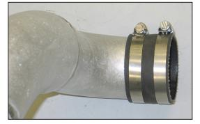
15. Install the provided silicone hose (08727) onto the K&N<sup>®</sup> intake tube and secure with the provided hose clamp.
