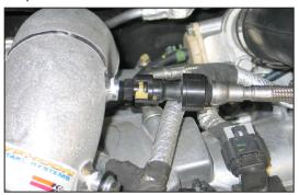
21. Connect the crank case vent hose to the quick connect fitting on the K&N $^{\circ}$  intake tube.
