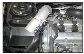
20. Install the K&N<sup>®</sup> intake tube into position on the turbo inlet and align with the tube mounting bracket. Secure the intake tube with the provided hose clamp and hardware.
