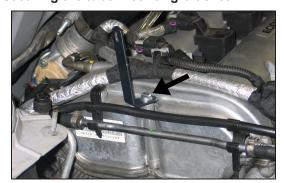
10a. On vehicles not equipped with a valve cover mounted engine id plate, install the tube mounting bracket assembly onto the engine and secure it with the provided hardware. Reinstall the bypass hose assembly back into the mounting boss. **NOTE: Be sure to apply the provided thread locking compound to the threads of the bolt securing the tube moutning bracket**.
