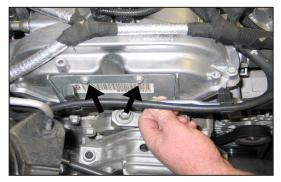
9. Lift the bypass hose assembly up to release it from mounting boss and then on vehicles equipped with an engine id plate, remove the two bolts shown. **NOTE: These bolts will not be reused.**
