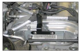
10.On vehicles equipped with a valve cover mounting engine id plate, install the tube mounting bracket (083123) onto the engine and secure it with the provided hardware. Reinstall the bypass hose back into the mounting boss.
