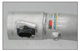
14. Install the mass air sensor into the K&N<sup>®</sup> intake tube and secure with the provided hardware.
