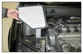
6. Pull up the lower air box to release it from the mounting gourmet and then remove the lower air box from the vehicle.
