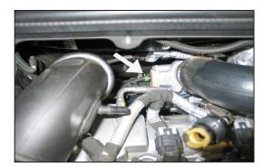
7. Loosen the hose clamp which secures intake tube to the turbo inlet.
