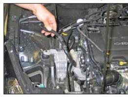
6. Unhook the two clips that secure the airbox drain tube to the inner fender, and then remove the drain tube from the vehicle.
