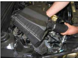
5. Lift the airbox assembly to dislodge it from the mounting grommets and then remove the airbox from the vehicle.
