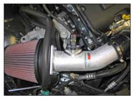
18. Connect the mass air sensor electrical connection.
