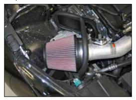
17. Install the K&N® air filter onto the filter adapter and secure with the provided hose clamp. NOTE: Drycharger® air filter wrap; part # RU-5147DK is available to purchase separately. To learn more about Drycharger® filter wraps or look up color availability please visit
