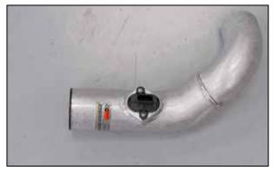
14. Install the mass air sensor into the K&N® intake tube and secure with the provided hardware.
