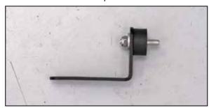
15. Install the rubber mounted stud onto the mounting bracket (010031A) and secure with the provided hardware.
