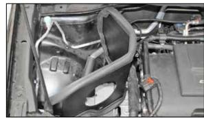
8. Install the heat shield assembly onto the engine mount and secure with the bolt removed in step #5. **NOTE: Do not completely tighten at this time.**
