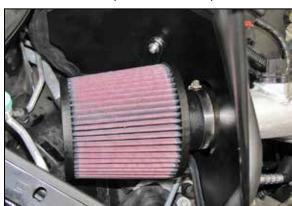
18. Install the K&N® air filter and secure with the provided hose clamp.
