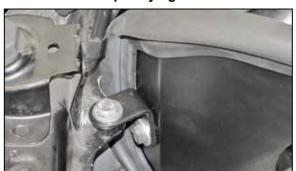
9. Install the provided "L" bracket (070066A) onto the core support and heat shield as shown using the provided hardware, then tighten all of the heat shield mounting hardware.
