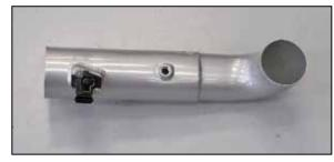
20. Install the mass air sensor into the K&N  $^{\! \rm 8}$  intake tube and secure with the provided hardware.
