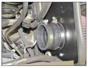
18. Install the provided hose (08051) onto the filter adapter and secure with the provided hose clamps.
