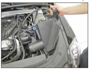
8. Pull up the coolant hoses from the air box and then remove the air box from the vehicle.
