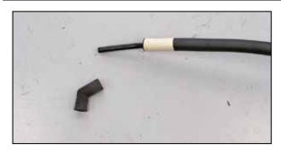
23. Remove the crank case vent tube coupler from the vent tube as shown.
