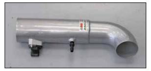
21. Install the provided crank case vent into the  $K\&N^{\circ}$  intake tube as shown.
