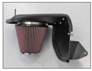
14. Install the K&N® air filter onto the filter adapter and secure with the provided hose clamp.
