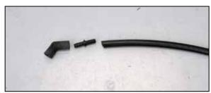
24. Install the union fitting into the coupler and then attach the provided crank case vent hose to the union.
