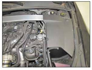
27. Reinstall the strut tower cover and snap it to the stand-off attached to the heat shield.
