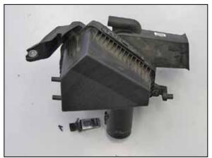
19. Remove the mass air sensor from the factory air box.
