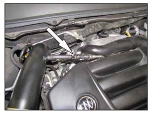
21. Reconnect crankcase vent line as shown.
