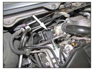
8. Install hose (084016) onto turbo inlet. Secure with provided hose clamp.
