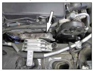
15. Remove forward motor mount bolt shown. **NOTE: Bolt will be reused.**
