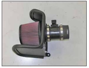
14. Install hose (084031) onto mass air housing and secure with provided hose clamp as shown.
