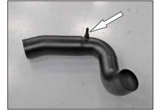
17. Install 3/8 barbed NPT fitting onto intake tube as shown.
