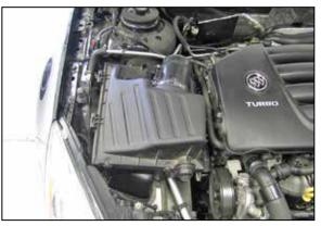
6. Lift up the air box to dislodge it from the mounting grommets; then remove from vehicle. **NOTE: K&N Engineering, Inc., recommends that customers do not discard factory air intake.**
