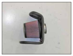
12. Insert filter through heat shield opening as shown.
