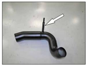
19. Install hose assembly onto intake tube as shown.
