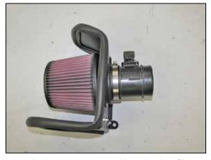
13.Install mass air sensor and housing into filter as shown and secure with the provided hose clamp. **NOTE: The arrow on the mass air housing indicating air flow should point away from filter.**
