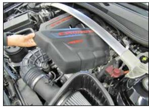
4. Lift up and remove the driver's side engine cover.
