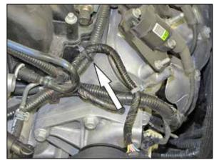
21. Connect the mass air sensor electrical connection and then secure the wiring harness to the engine harness with the provided tie wrap.
