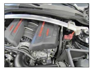
22. Reinstall the driver's side engine cover.
