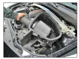
7. Lift up the air filter housing to dislodge it from the inner fender and then remove it from the vehicle.
