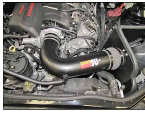
19. Install the intake tube into the Hump hose and then into the hose at the throttle body, adjust the tube for best fit and then secure with the provided hose clamps.
