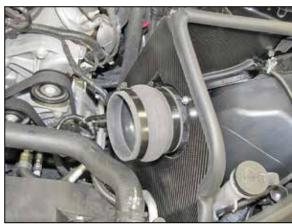
15. Install the provided hump coupler hose #08418 onto the filter adapter and secure with the provided hose clamp.
