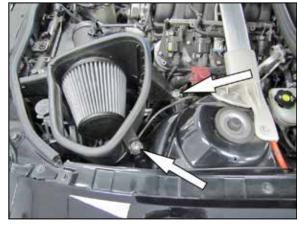
6. Remove the two nuts securing the air filter housing to the inner fender.
