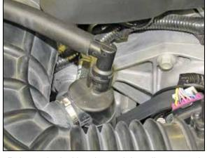
3. Release the locking ring and then disconnect the crank case vent from the intake tube.
