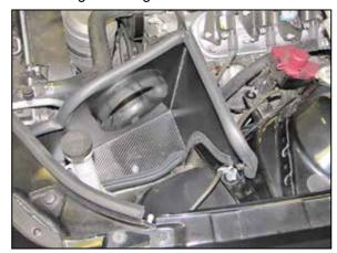
13. Install the heat shield assembly into the vehicle so that the mounting bracket slides onto the mounting stud and the mounting stud inserts into the factory mounting bracket. Then secure the heat shield with the factory nut and secure the ground strap to the threaded stud with the factory fastener.
