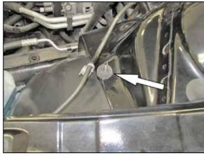
12. Install the provided rubber washer onto the air filter housing mounting stud as shown.
