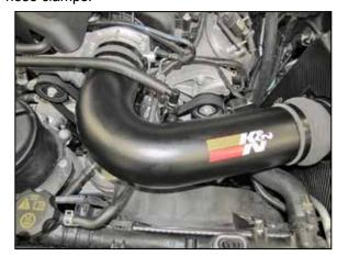
20. Connect the stock ccv hose the quick disconnect fitting installed into the intake tube.
