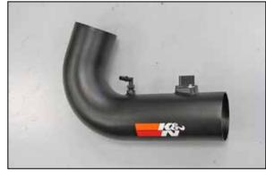
18. Install the 90° NPT quick disconnect npt fitting into the K&N® intake tube as shown.
