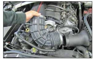
5. Loosen the hose clamps securing the intake tube to the throttle body and mass air sensor then remove the intake tube from the vehicle.
