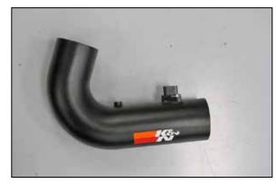
17. Install the mass air sensor into the K&N<sup>®</sup> intake tube and secure with the provided hardware.
