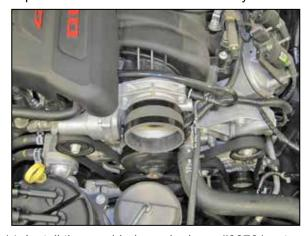
14. Install the provided coupler hose #08761 onto the throttle body and secure with the provided hose clamp.
