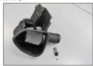
16. Remove the mass air sensor from the factory housing as shown.
