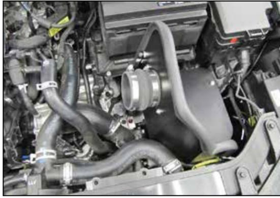
12. Install the provided coupler hose (087121) onto the filter adapter and secure with the provided hose clamp.
