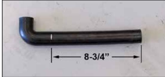
13. Measure 8-3/4" from the end of the provided air injection hose and then cut the hose.
