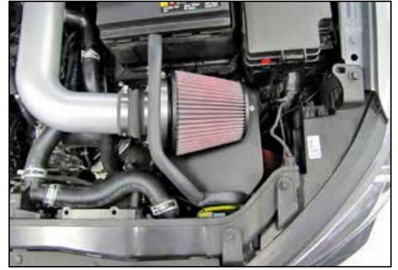
18. Install the K&N® air filter onto the filter adapter and secure with the provided hose clamp.
