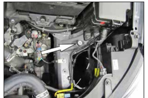
6. Install the provided rubber mounted stud into the air filter mounting location on the inner fender as shown.
