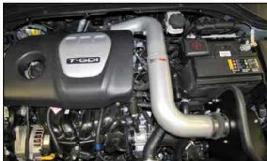
16. Install the K&N® intake tube assembly into the coupling hose at the turbo and then into the coupling hose at the filter adapter, adjust the tube for best fit and then secure with the provided hose clamps.
