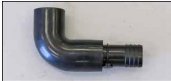
14. Install the provided union into the 90° portion of the cut crank case vent hose as shown.
