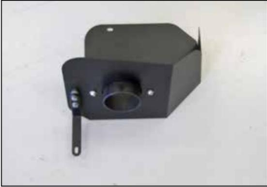
8. Install the provided "L" bracket (064347) onto the heat shield using the provided spacers and hardware.
