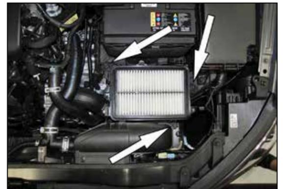
5. Remove the three bolts that secure the lower air filter housing to the inner fender and then remove the lower housing from the vehicle.
