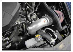
16. Install the driver side intake tube (27677) into the coupler at the turbo and then into the coupler at the filter adapter, adjust the tube and heat shield assembly for best fit and then secure with the provided hose clamps. 21. Install the passenger side heat shield assembly into the vehicle so the fresh air intake inserts into the opening of the heat shield and then secure the heat shield with the provided hardware.
