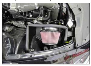
shown and secure the adapter with the provided hardware.
