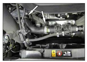
7. Release the spring clamps that secure the passenger side BOV hose to the BOV and intake tube, then remove the passenger side BOV hose. **NOTE: This hose will be reused.**
