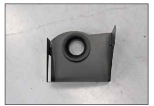
10. Install one of the two provided filter adapters into the driver side heat shield (073252) as
