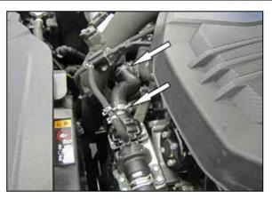
24. Install the passenger side intake tube (27678) into the coupler at the turbo and then into the coupler at the filter adapter, adjust the tube and heat shield assembly for best fit and then secure with the provided hose clamps. Install the driver side BOV hose onto the fitting on the K&N<sup>®</sup> intake tube and then onto the BOV valve. Secure with the factory spring clamps.
