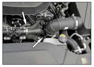
4. Release the spring clamps that secure the driver side BOV hose to the BOV and intake tube, then remove the driver side BOV hose. **NOTE: This hose will be reused.**  side air filter housing to the inner fender, loosen the hose clamp that secures the intake tube to the air filter housing and disconnect the tube. Remove the driver side air filter housing from the vehicle. **NOTE: K&N Engineering, Inc., recommends that customers do not discard factory air intake.**
