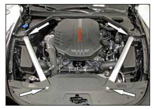
2. Remove the four bolts shown that secure the two strut tower braces to the vehicle and then remove the braces from the vehicle. **NOTE; These braces and bolts will be reinstalled later.**  vent lines attached to the driver's side intake tube and then disconnect the vent lines from the intake tube.
