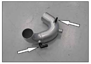
15. Install the NPT vent fittings into the driver side  $K\&N^{\circ}$  intake (27677) as shown.
