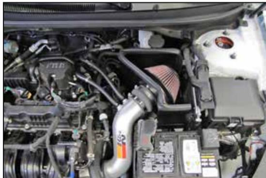
13. Connect the factory vent lines to the hoses connected to the K&N® intake tube.
