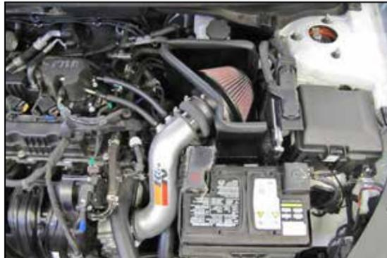
12. Using the provided coupler hose (084079) Install the K&N® intake tube into the vehicle, adjust the tube for best fit and then secure with the provided hose clamps.
