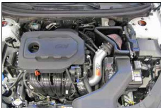
14. Reinstall the decorative engine cover. Install the factory fresh air intake duct into the K&N® heat shield and core support.
