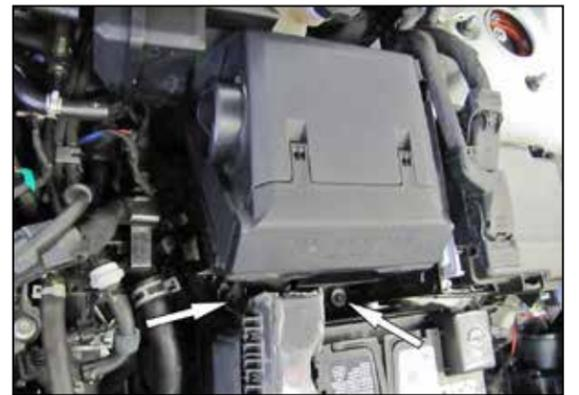
5. Remove the two bolts that secure the factory air filter housing and then lift to remove the factory air filter housing from the vehicle.
