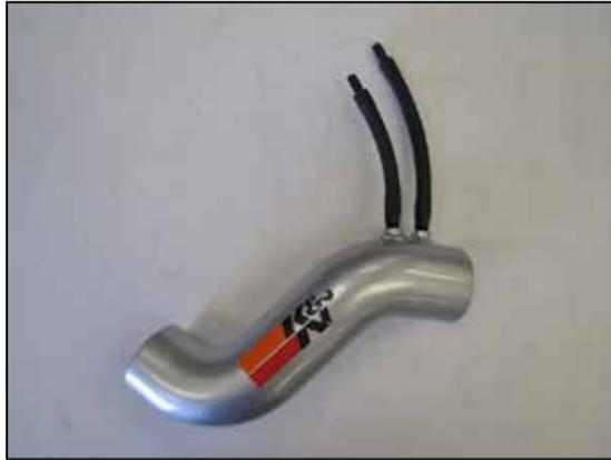
11. Assemble the K&N® intake tube, Breather hoses and fittings as shown.
