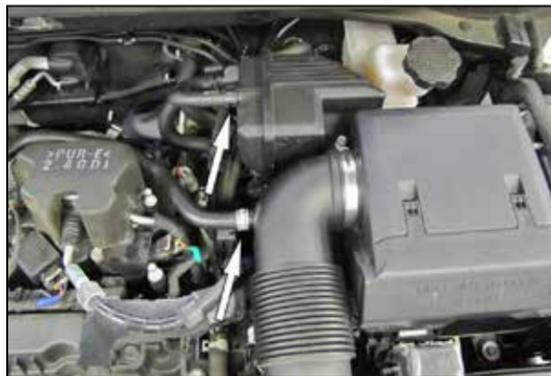
3. Disconnect the breather hoses from the factory intake tube and the intake plenum.
