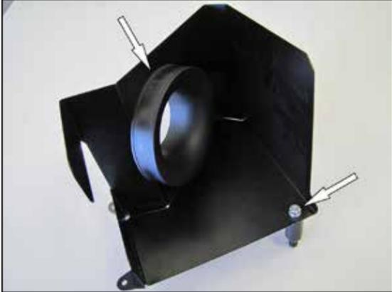
8. Install the filter adapter into the heat shield and secure with the provided hardware. Install the heat shield mount onto the heat shield using the provided hardware.
