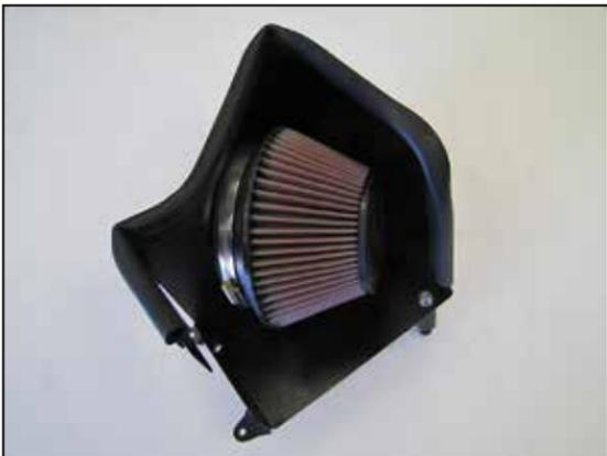
9. Install the provided edge trim onto the heat shield as shown, then install the K&N® air filter onto the filter adapter and secure with the provided hardware.
